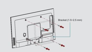
To prevent internal damage to the TV and ensure the TV is mounted securely, be sure to use fixing screws (not provided) which are 9.5-12.5mm in length. t-----'
