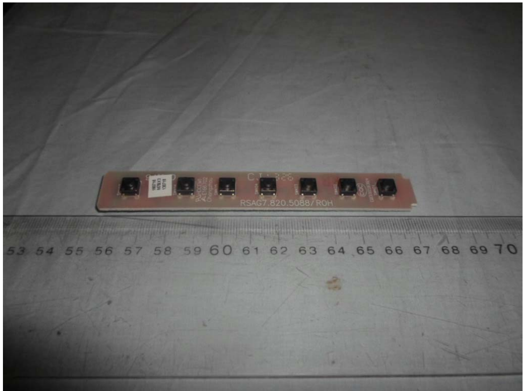
FIGURE 11 LED LCD TV (M/N: LHD32A300MUS) KEY BOARD (COMPONENT SIDE)
