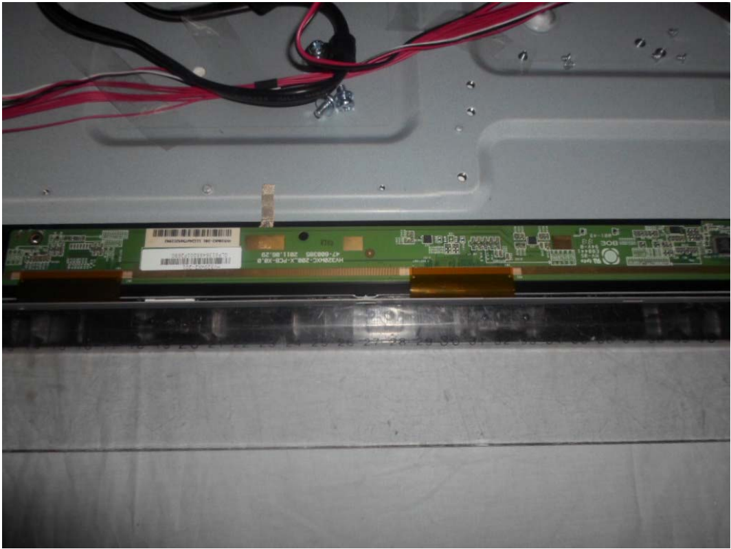
FIGURE 13 LED LCD TV (M/N: LHD32A300MUS) LCD PANEL CONTROL BOARD (COMPONENT SIDE #1)
