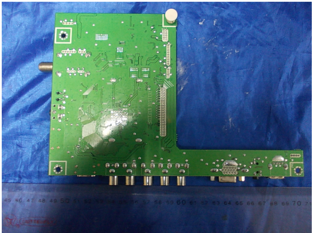
FIGURE 6 LED LCD TV (M/N: LHD32A300MUS) MAIN BOARD (SOLDERED SIDE)
