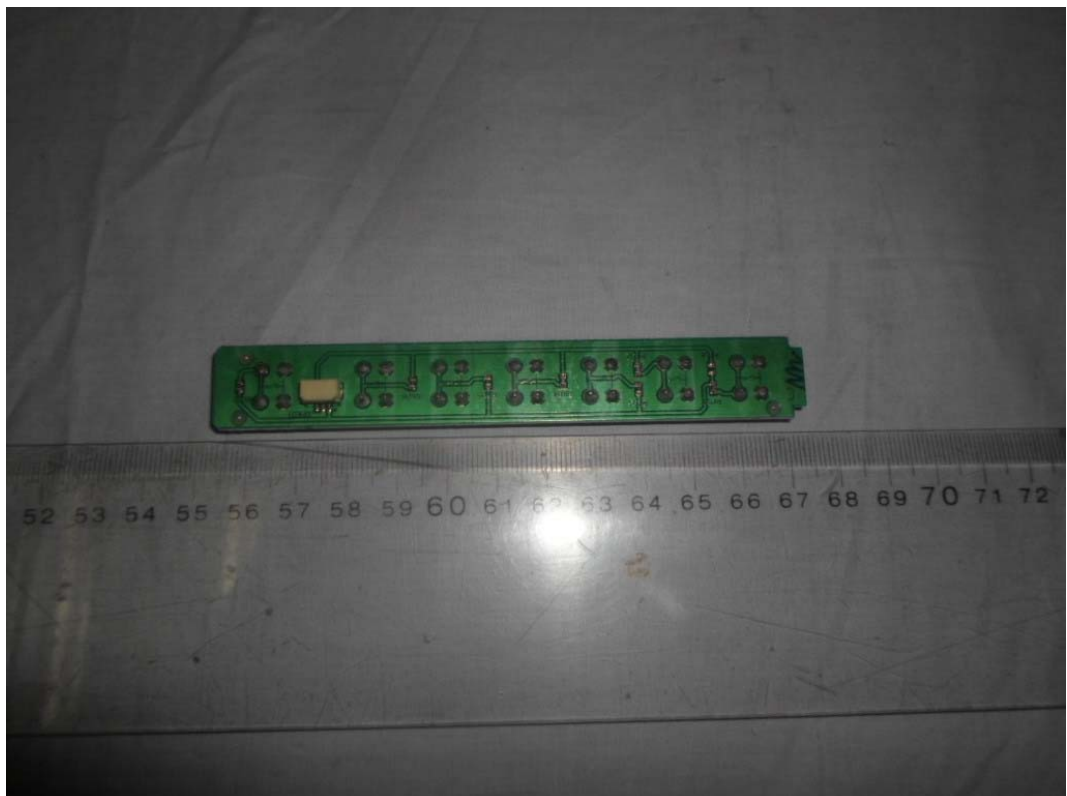
FIGURE 12 LED LCD TV (M/N: LHD32A300MUS) KEY BOARD (SOLDERED SIDE)
