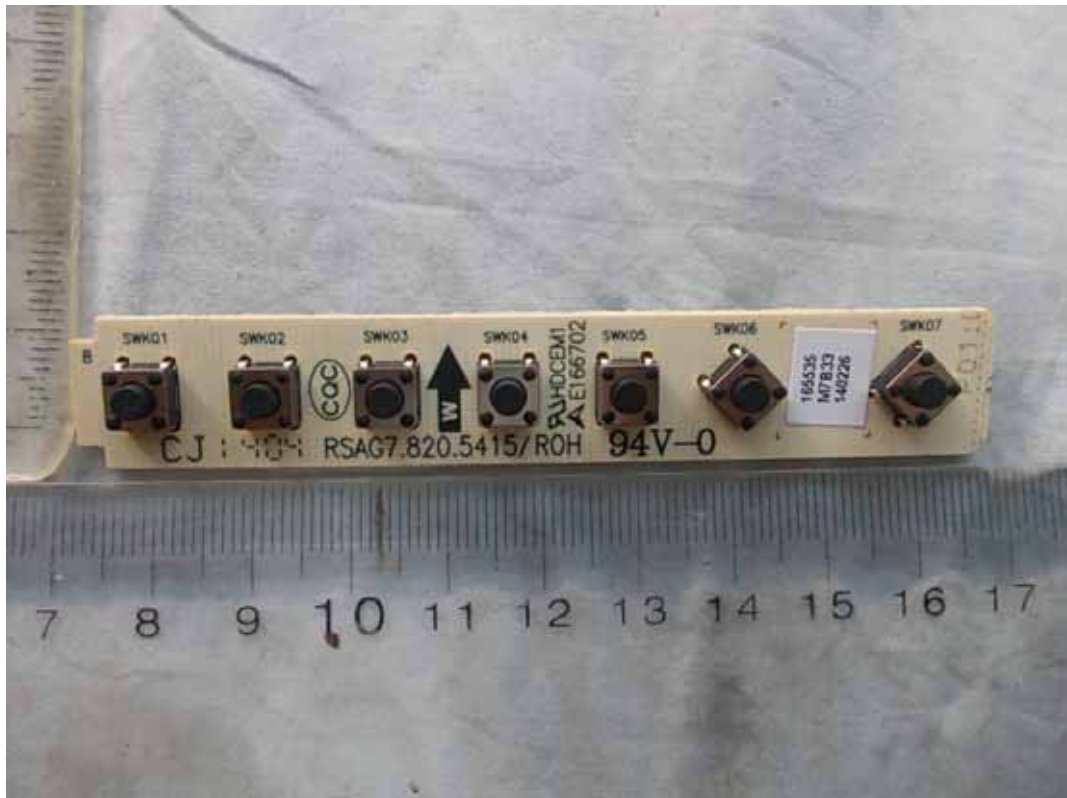
FIGURE 10 LED LCD TV (M/N: LHD32K20DWUS) KEY BOARD (COMPONENT SIDE)
