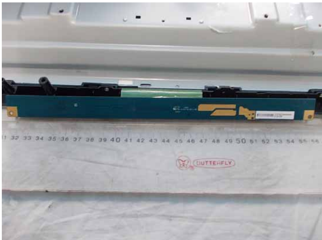
FIGURE 15 LED LCD TV (M/N: LHD32K20DWUS) LCD PANEL CONTROL BOARD (SOLDERED SIDE)
