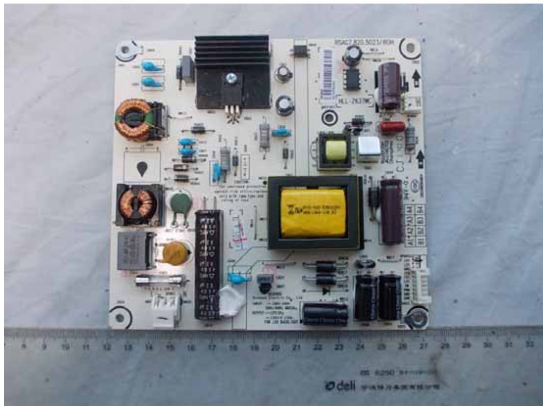
FIGURE 3 LED LCD TV (M/N: 32K366MH) POWER BOARD (COMPONENT SIDE)
