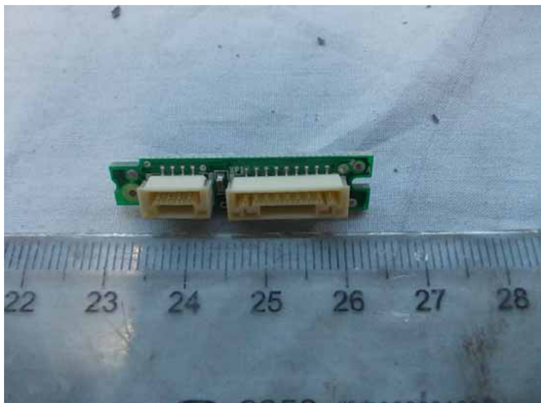
FIGURE 15 LED LCD TV (M/N: 32K366MH) IR BOARD (SOLDERED SIDE)
