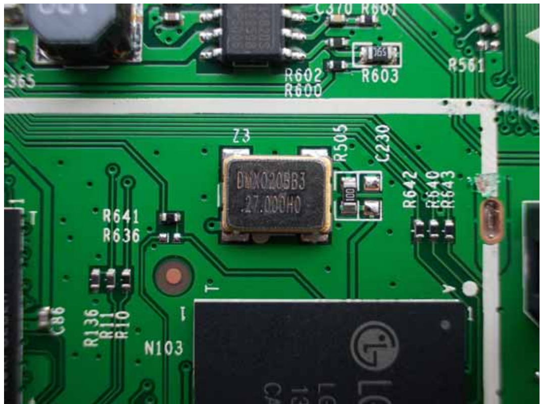
FIGURE 11 LED LCD TV (M/N: 32K366MH) CRYSTAL #3 ON MAIN BOARD
