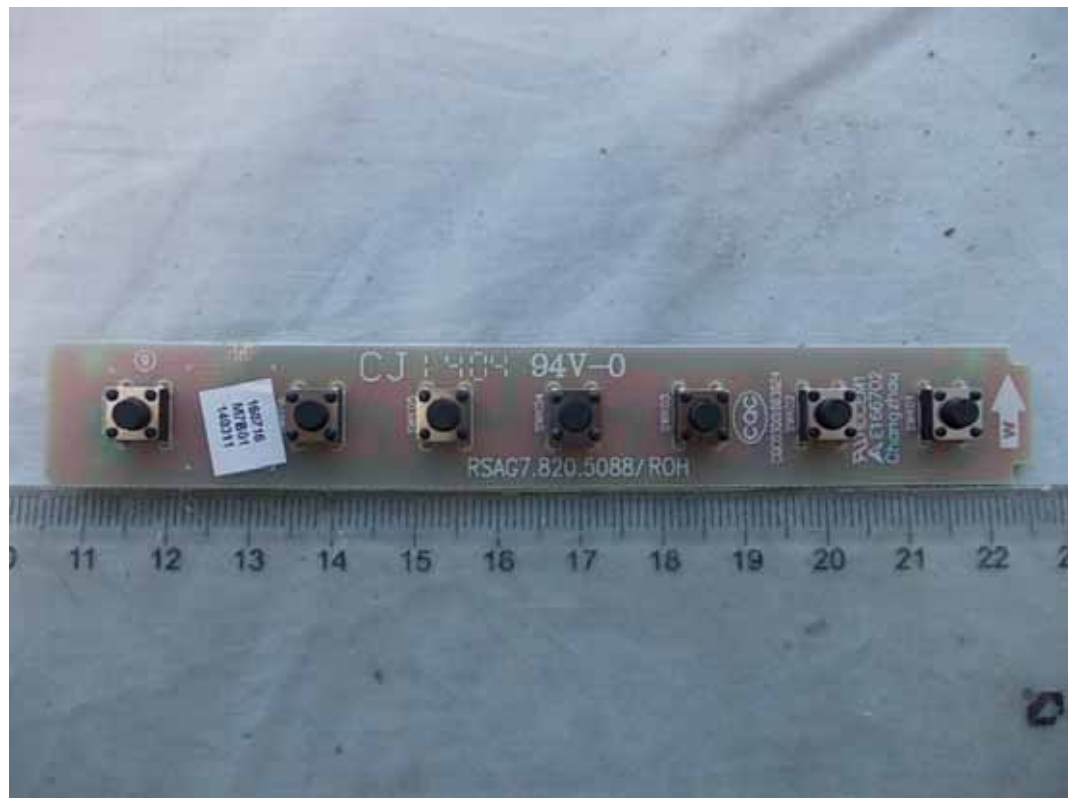
FIGURE 12 LED LCD TV (M/N: 32K366MH) KEY BOARD (COMPONENT SIDE)
