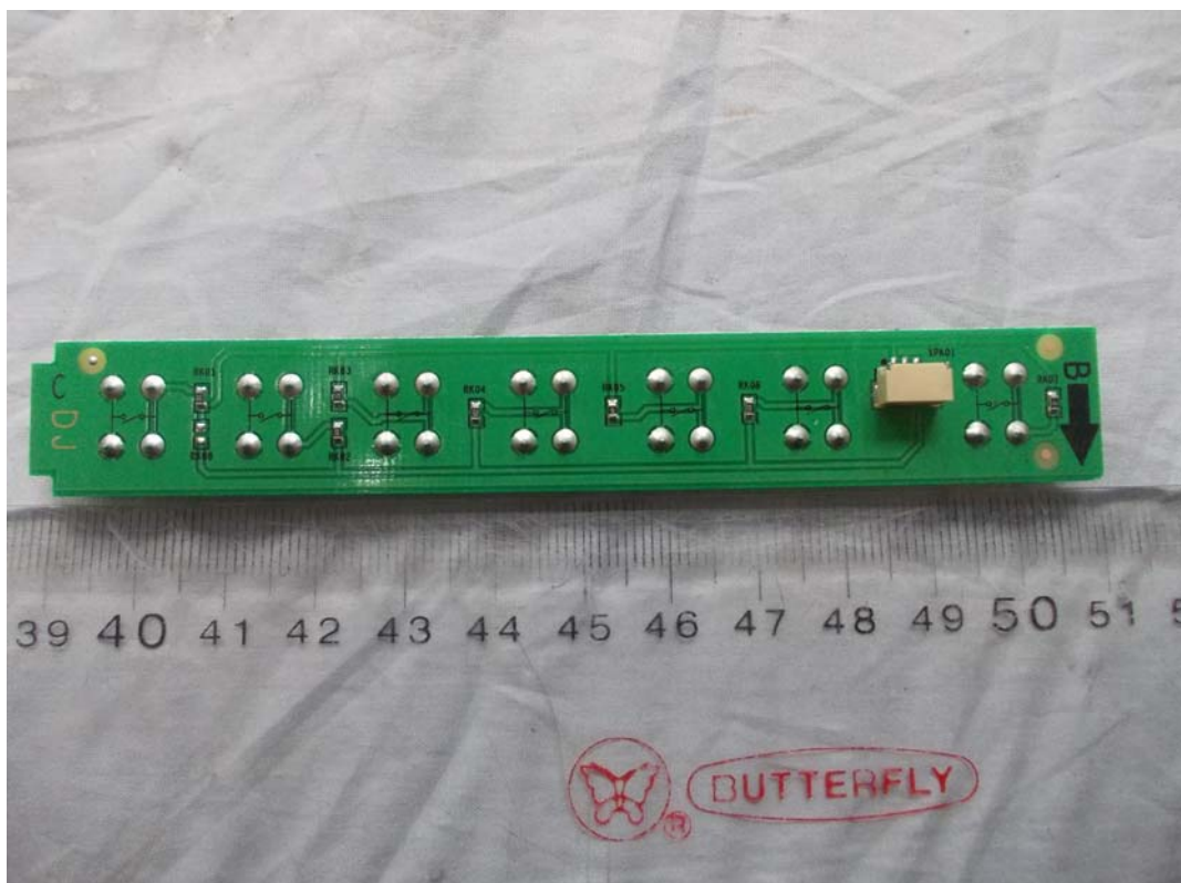
FIGURE 10 LED LCD TV (M/N: 32K366HS) KEY BOARD (SOLDERED SIDE)
