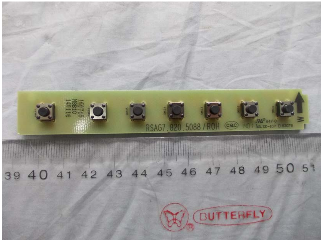
FIGURE 9 LED LCD TV (M/N: 32K366HS) KEY BOARD (COMPONENT SIDE)
