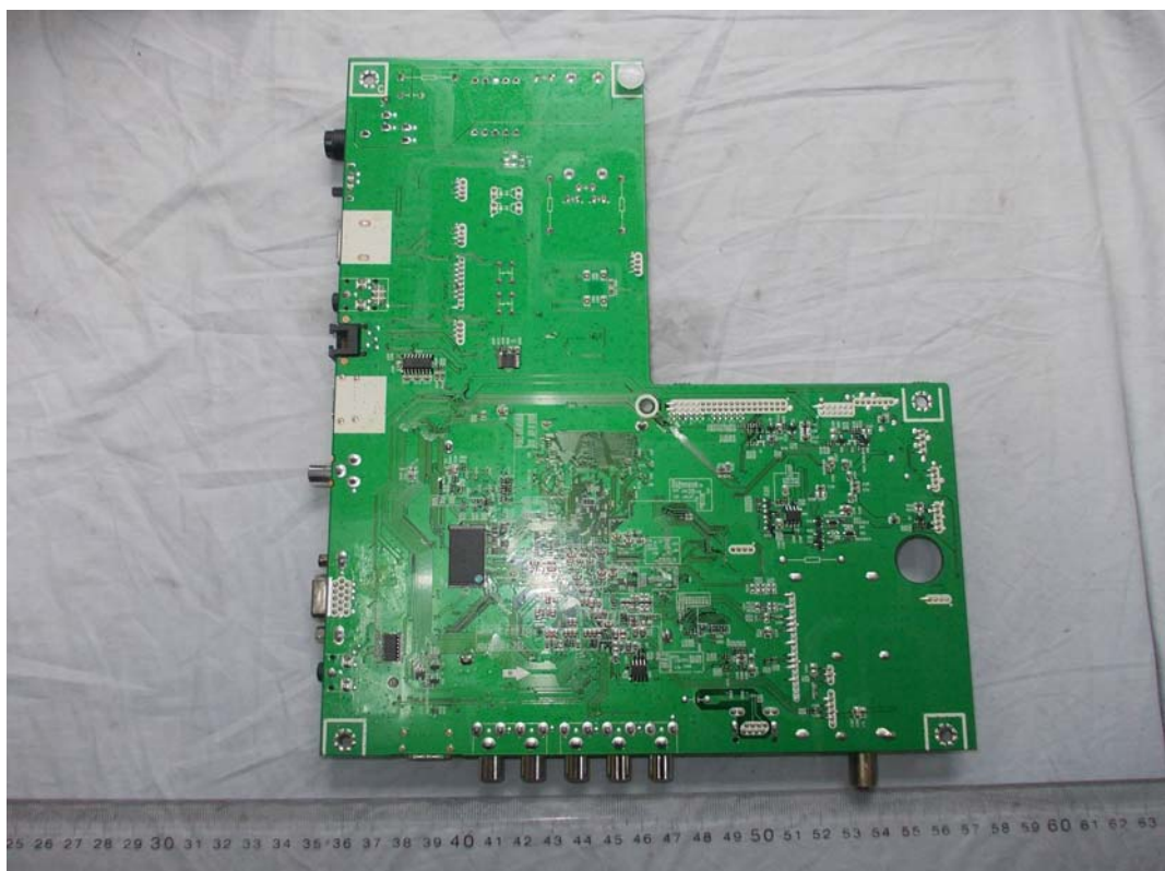
FIGURE 6 LED LCD TV (M/N: 32K366HS) MAIN BOARD (SOLDERED SIDE)
