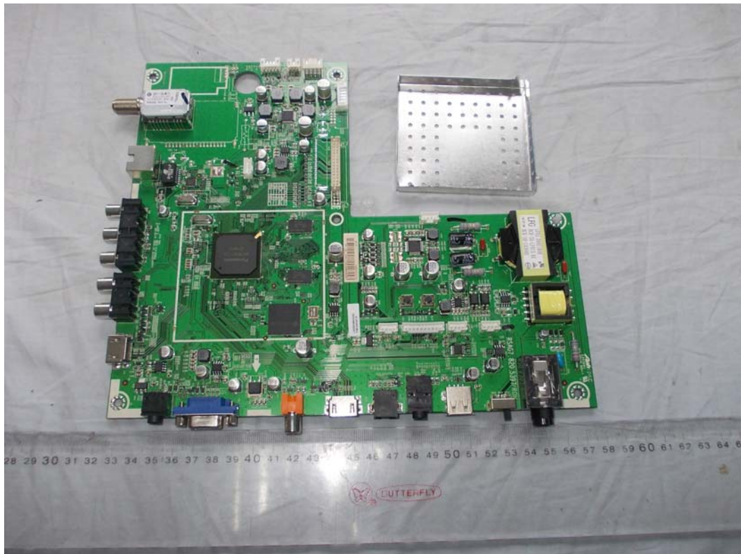
FIGURE 5 LED LCD TV (M/N: 32K366HS) MAIN BOARD (COMPONENT SIDE)
