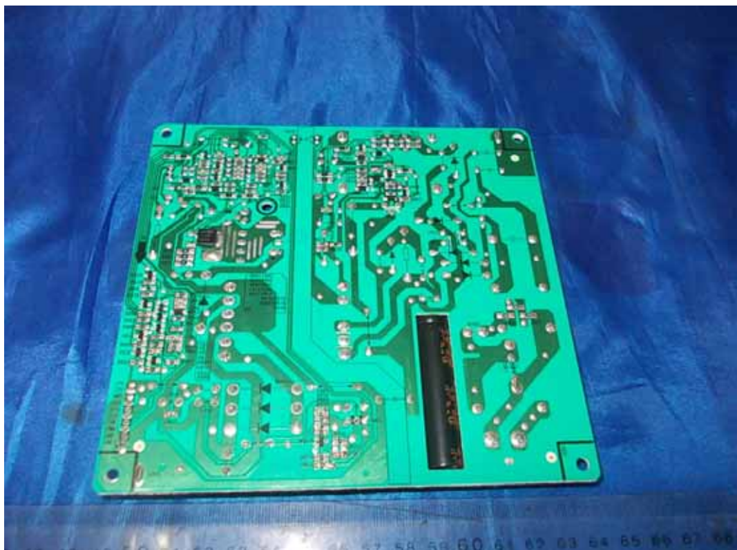
FIGURE 4 LED LCD TV (M/N: 32K366W) POWER BOARD (SOLDERED SIDE)
