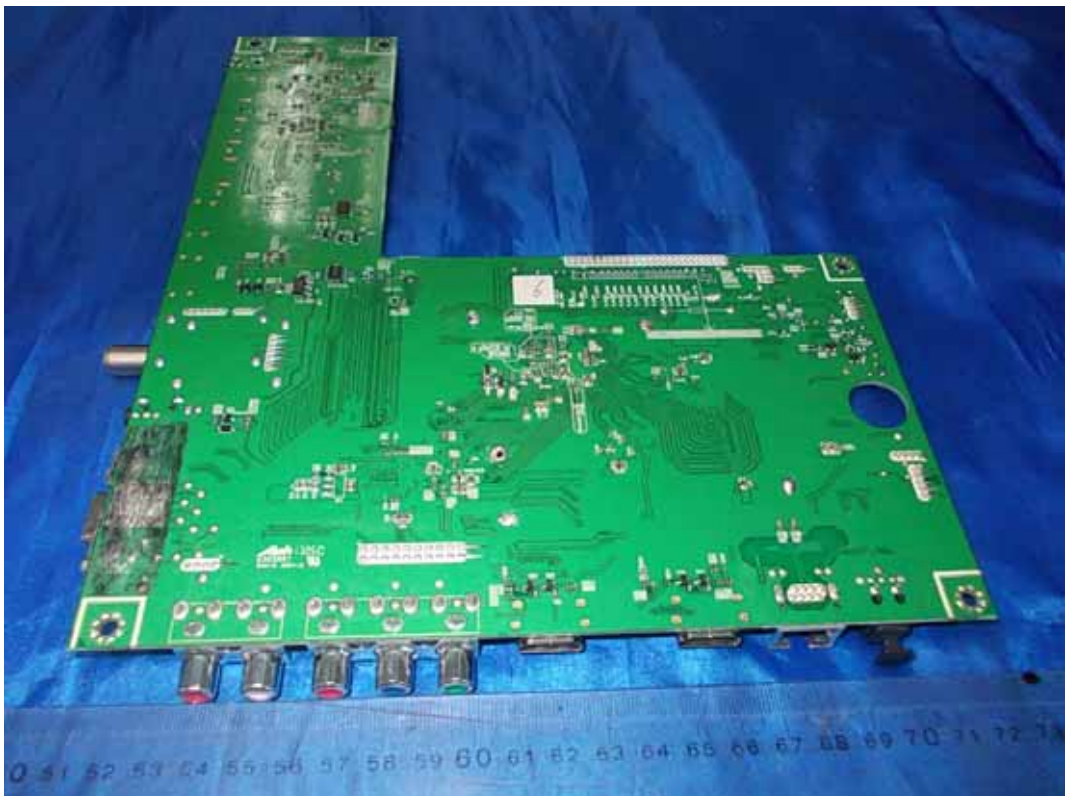
FIGURE 6 LED LCD TV (M/N: 32K366W) MAIN BOARD (SOLDERED SIDE)
