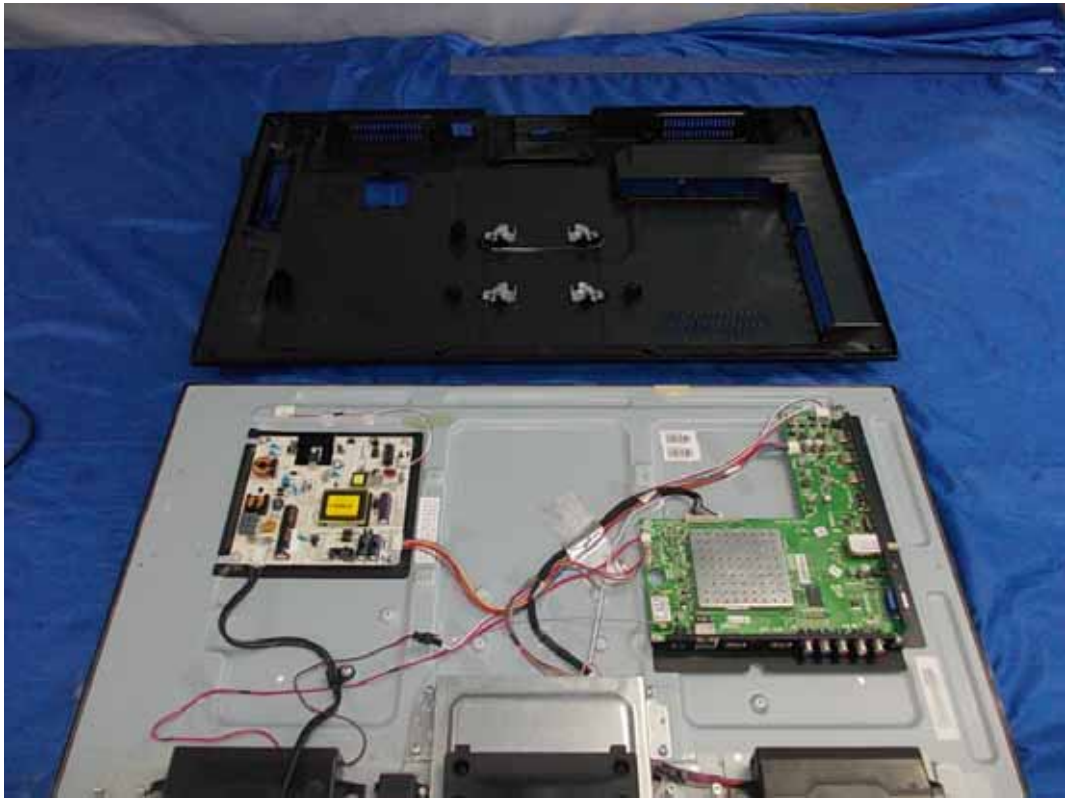
FIGURE 1 LED LCD TV (M/N: 32K366W) COVER REMOVED
