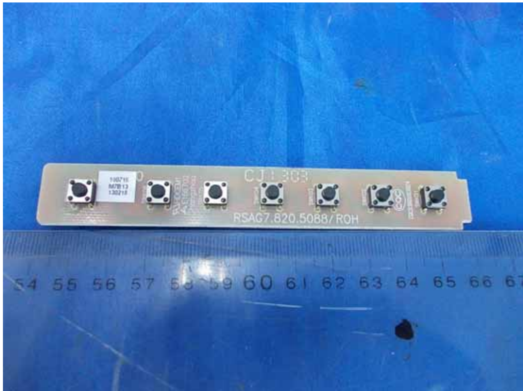
FIGURE 10 LED LCD TV (M/N: 32K366W) KEY BOARD (COMPONENT SIDE)
