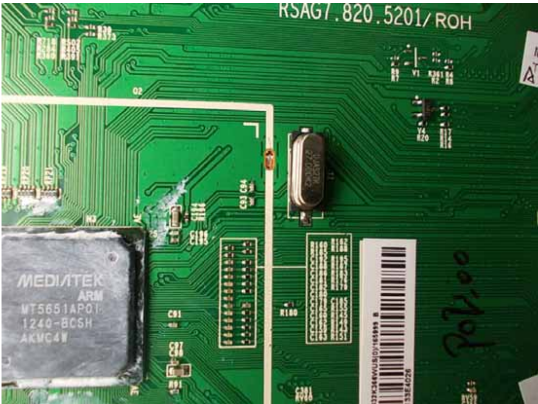
FIGURE 8 LED LCD TV (M/N: 32K366W) CRYSTAL ON MAIN BOARD
