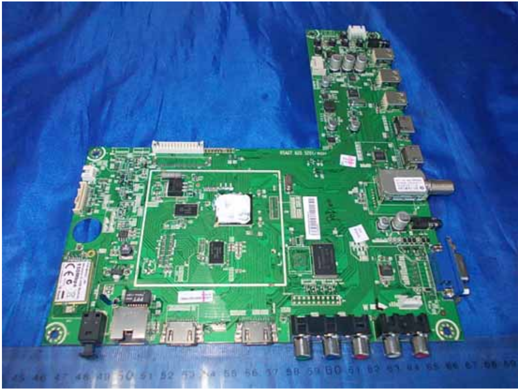
FIGURE 5 LED LCD TV (M/N: 32K366W) MAIN BOARD (COMPONENT SIDE)
