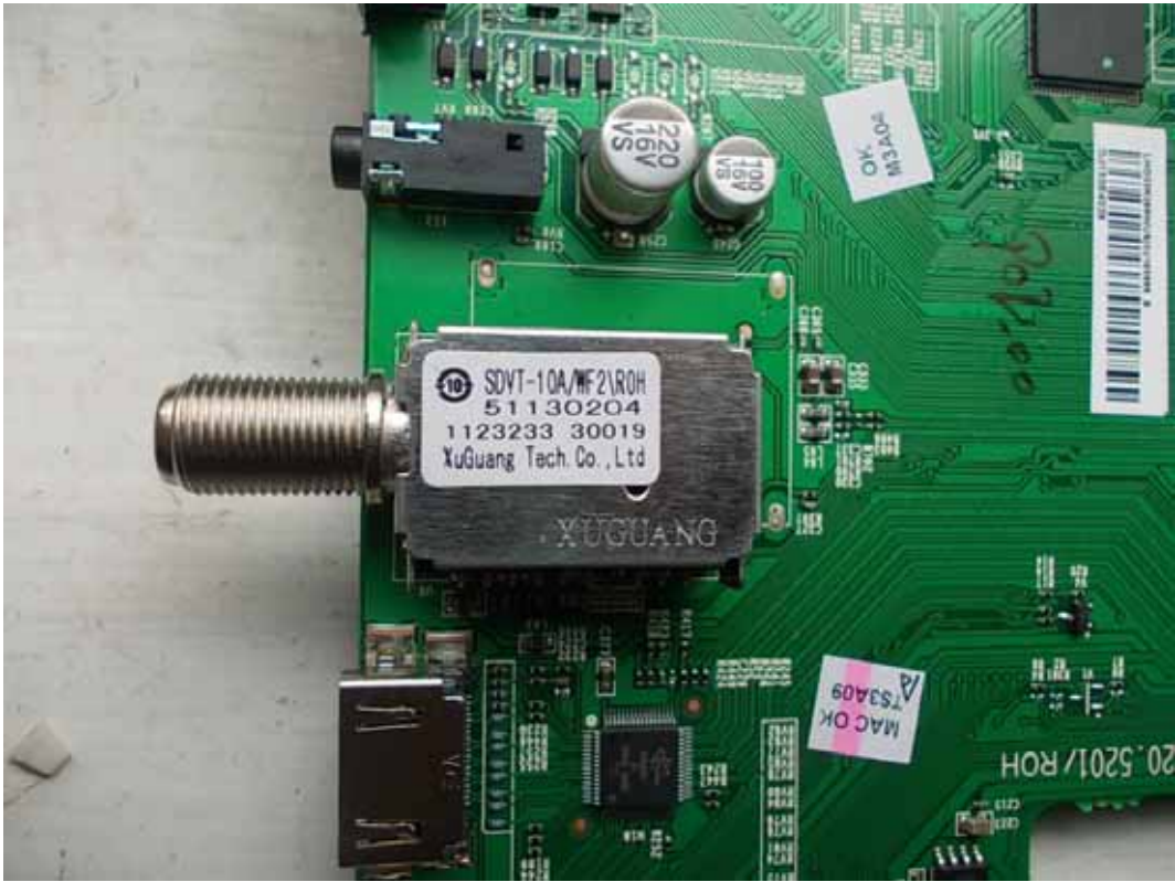
FIGURE 7 LED LCD TV (M/N: 32K366W) TUNER ON MAIN BOARD
