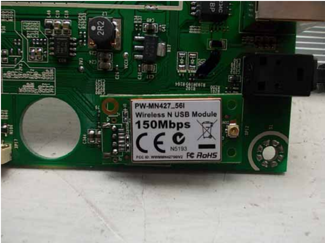
FIGURE 9 LED LCD TV (M/N: 32K366W) WIRELESS N USB MODULE
