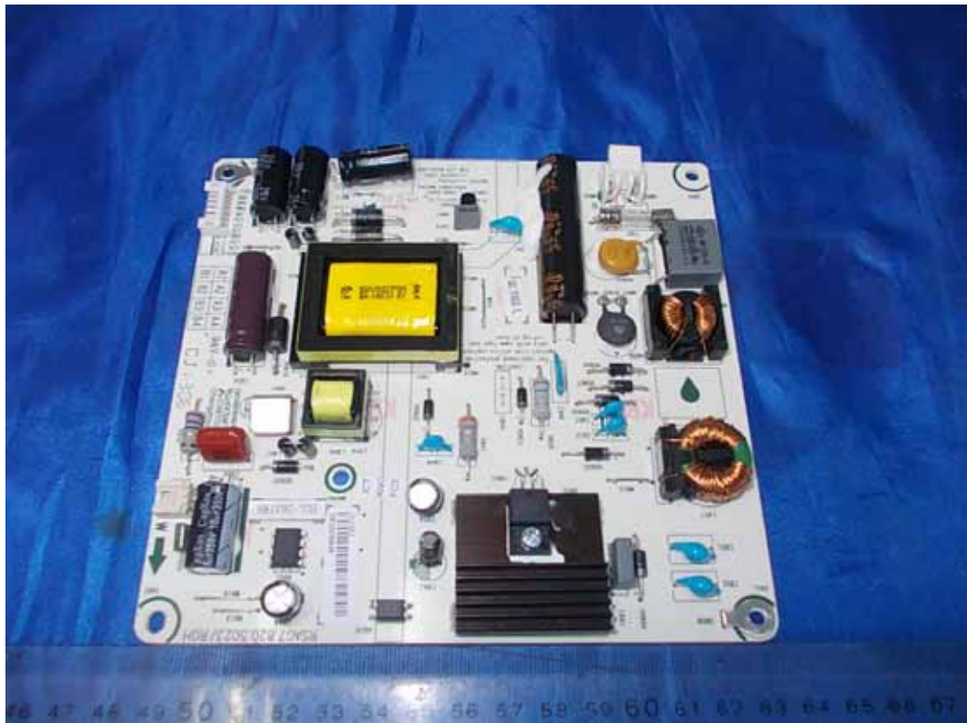
FIGURE 3 LED LCD TV (M/N: 32K366W) POWER BOARD (COMPONENT SIDE)
