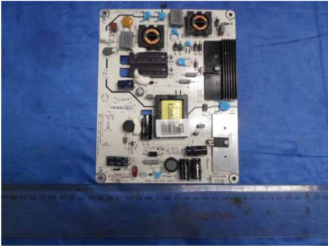
FIGURE 2 LED LCD TV (M/N: LHD32K310HUS) POWER BOARD (COMPONENT SIDE)
