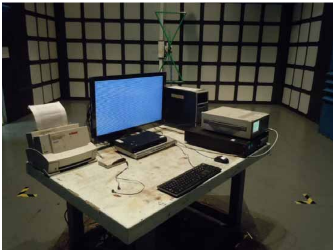
SETUP WITH MAXIMUM DETECTED EMISSION AT VERTICAL POLARIZATION (TEST MODE: HDMI 640*480@60Hz)
