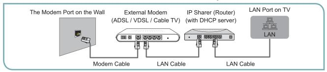
Depending on how your network is configured, you may be able to attach your TV to your LAN by connecting the LAN port on the back of your TV directly to a network wall outlet with a Cat 5 cable. See the diagram below. Note that the wall outlet is attached to a modem or router elsewhere in your house.
