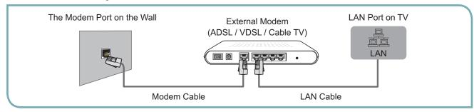
You can attach your TV to your LAN by connecting the LAN port on the back of your TV to an IP Sharer which is connected to an external modem. Use LAN cable for the connection. See the diagram below.
