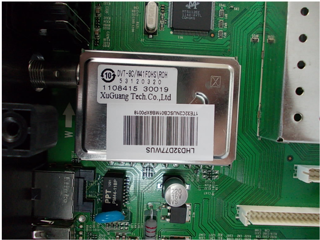
FIGURE 7 LED LCD TV (M/N: LHD32D77WUS) TUNER ON MAIN BOARD
