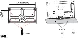
Be sure to follow the instructions, in correct installation of the stand (pedestal) may result in the TV falling over.
