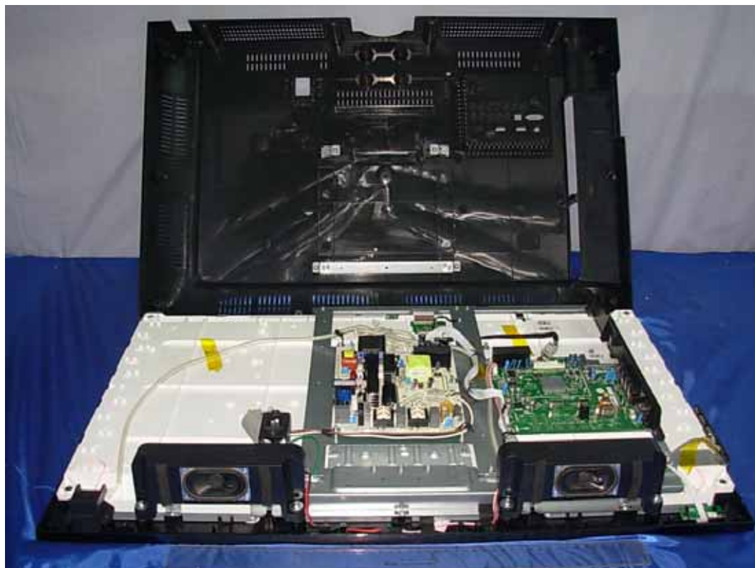
FIGURE 1 LCD TV (M/N: LHD32V77AUS) COVER REMOVED
