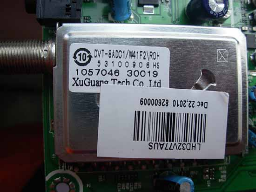
FIGURE 5 LCD TV (M/N: LHD32V77AUS) TUNER
