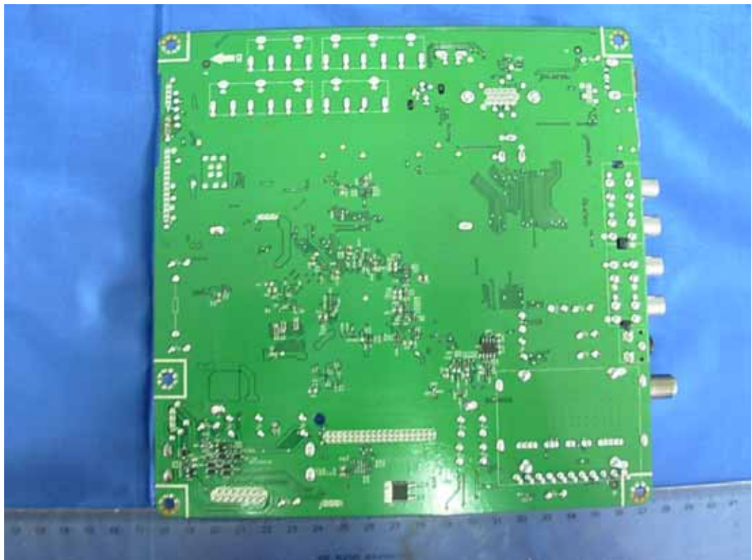
FIGURE 3 LCD TV (M/N: LHD32V77AUS) MAIN BOARD (SOLDERED SIDE)
