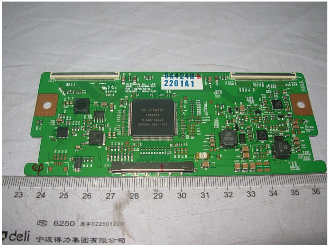
FIGURE 18 LCD TV (M/N: LTDN37W60MH) DISPLAY BOARD (COMPONENT SIDE)
