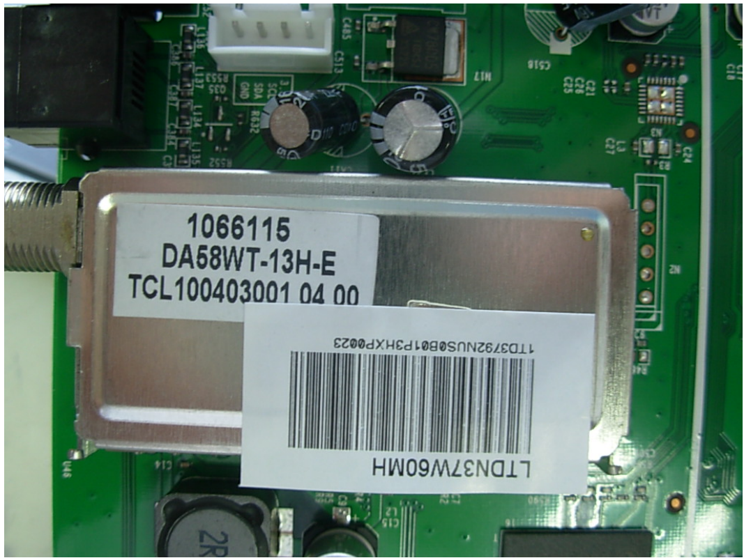
FIGURE 11 LCD TV (M/N: LTDN37W60MH) TUNER
