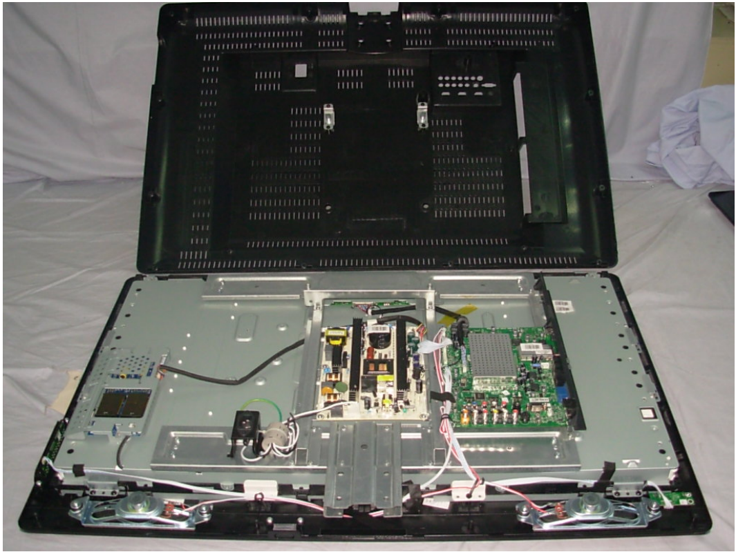
FIGURE 1 LCD TV (M/N: LTDN37W60MH) COVER REMOVED
