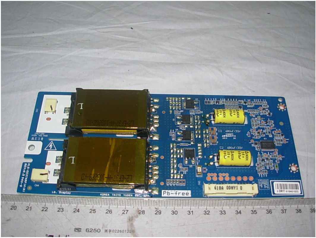
FIGURE 16 LCD TV (M/N: LTDN37W60MH) HIGH VOLTAGE SIGNAL BOARD (COMPONENT SIDE)
