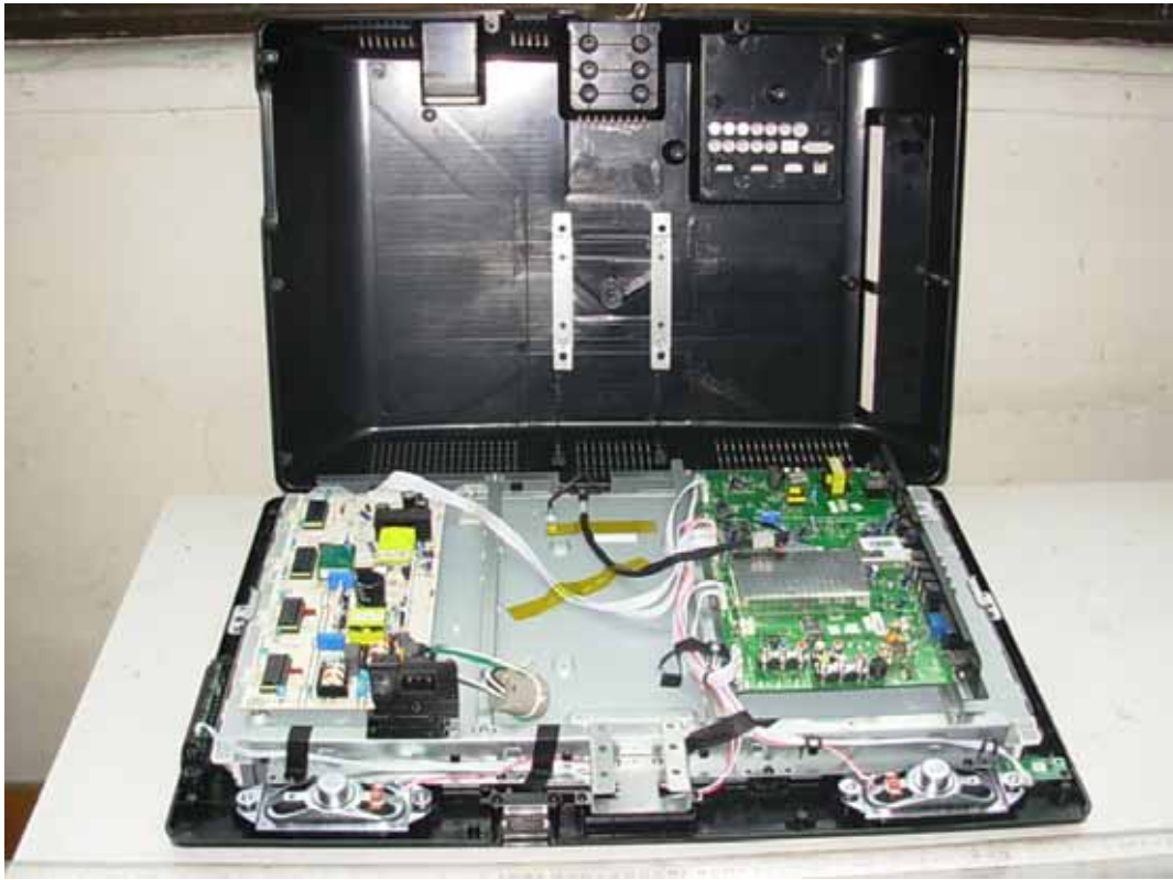
FIGURE 1 LCD TV (M/N: LTDN26W60HS) COVER REMOVED
