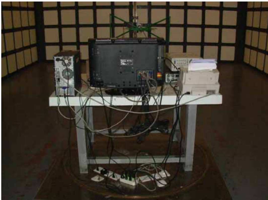
BACK VIEW OF RADIATED EMISSION TEST
