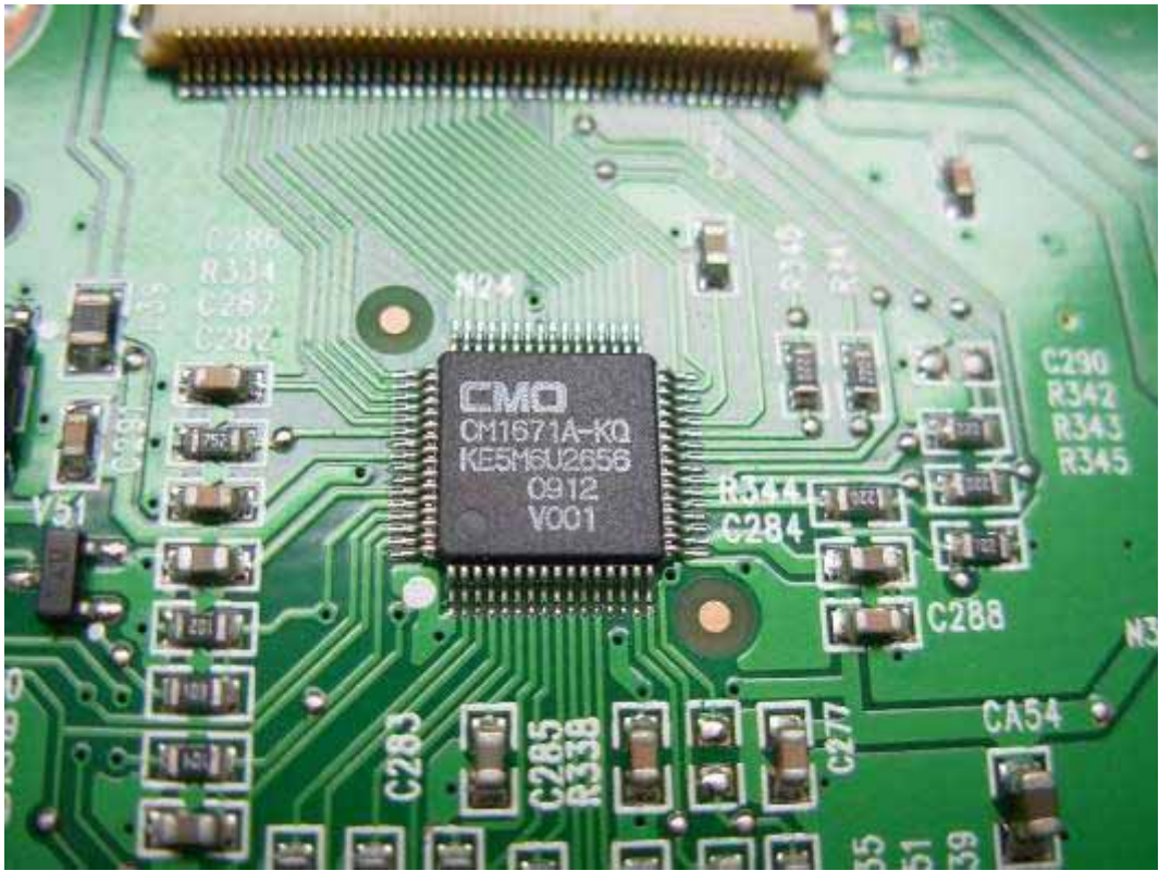
FIGURE 19 LCD TV (M/N: ELCHS262) CHIP ON LCD PANEL MAIN BOARD
