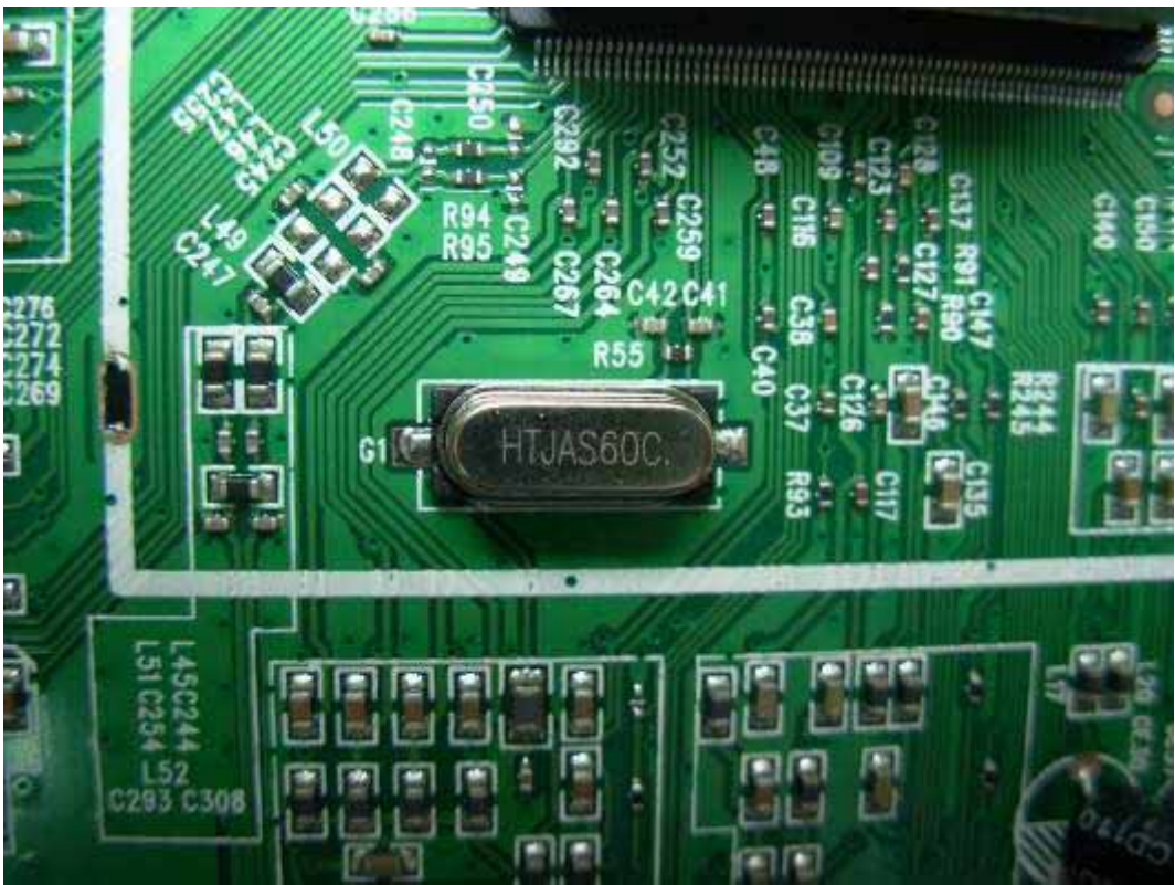
FIGURE 6 LCD TV (M/N: ELCHS262) CRYSTAL ON MAIN BOARD
