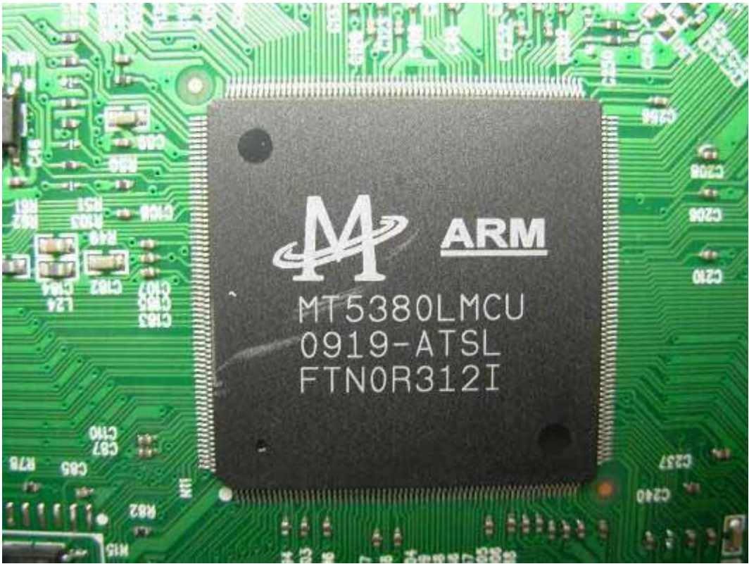
FIGURE 5 LCD TV (M/N: ELCHS262) CHIP ON MAIN BOARD
