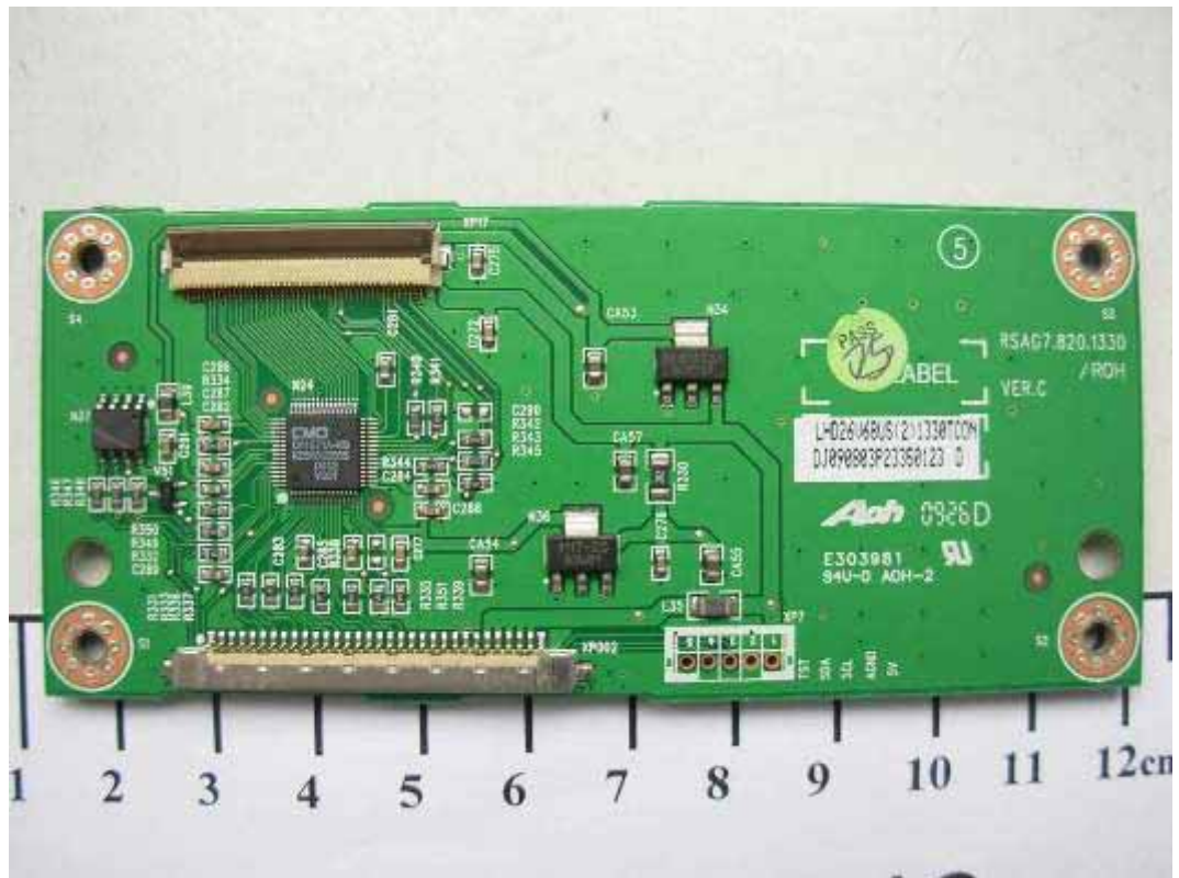
FIGURE 17 LCD TV (M/N: ELCHS262) LCD PANEL MAIN BOARD (COMPONENT SIDE)
