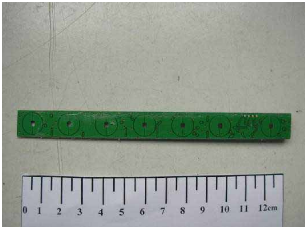
FIGURE 14 LCD TV (M/N: ELCHS262) KEY BOARD (SOLDERED SIDE)
