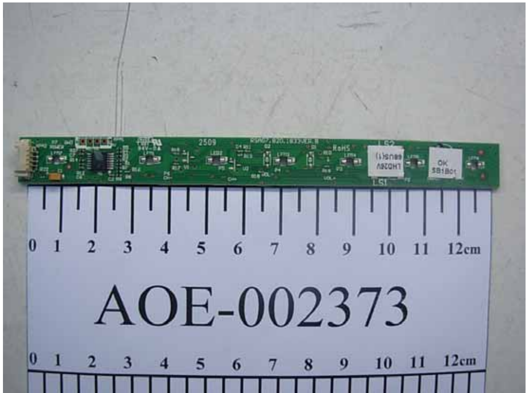
FIGURE 11 LCD TV (M/N: ELCHS262) BUTTON BOARD (COMPONENT SIDE)
