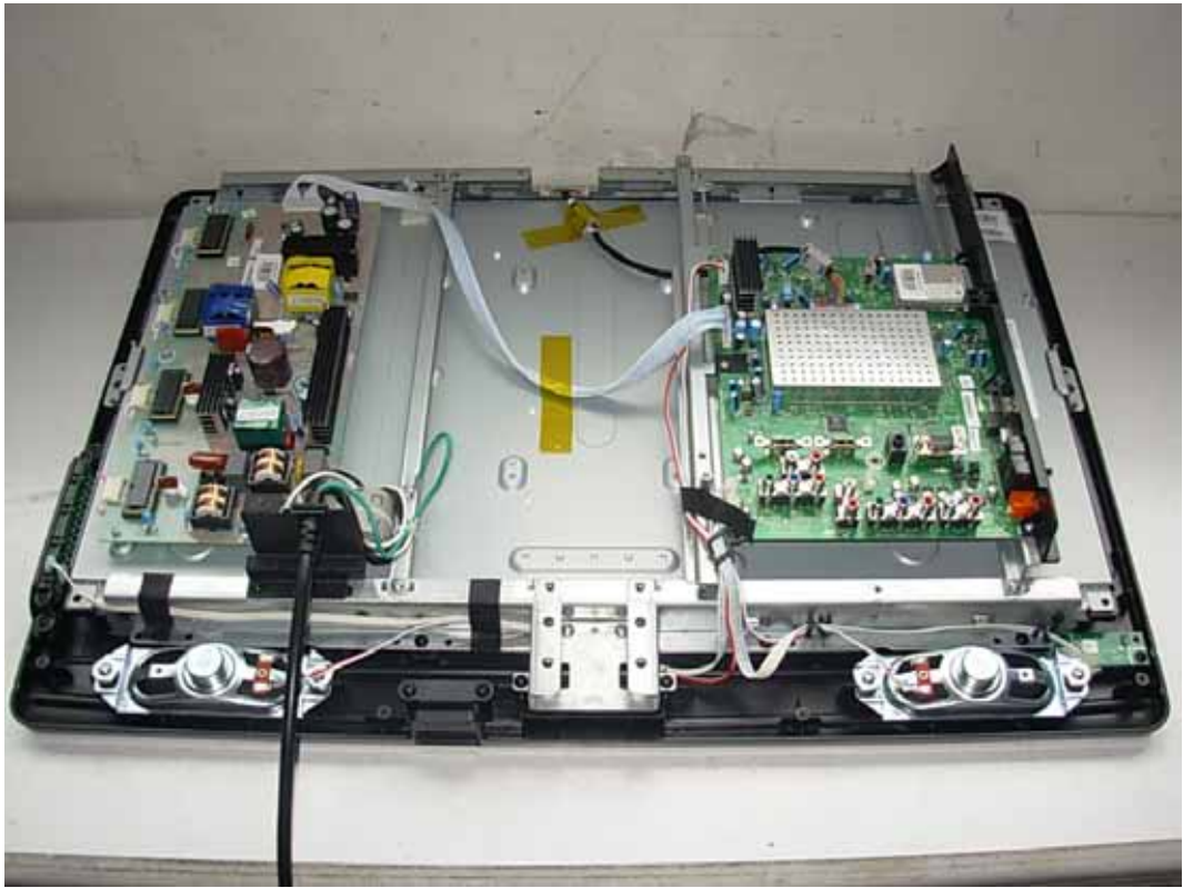
FIGURE 1 LCD TV (M/N: ELCHS262) COVER REMOVED
