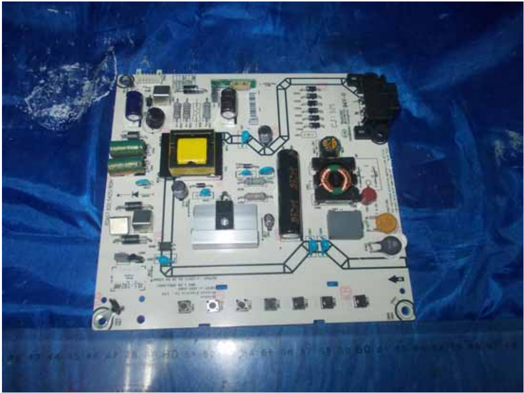
FIGURE 3 LED LCD TV (M/N: LHD23A300US) POWER BOARD (COMPONENT SIDE)
