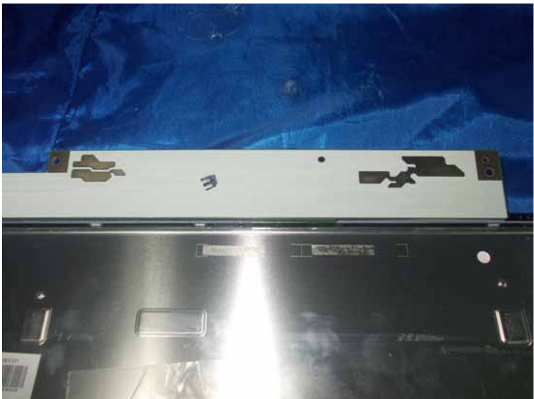
FIGURE 14 LED LCD TV (M/N: LHD23A300US) LCD PANEL CONTROL BOARD (SOLDERED SIDE)
