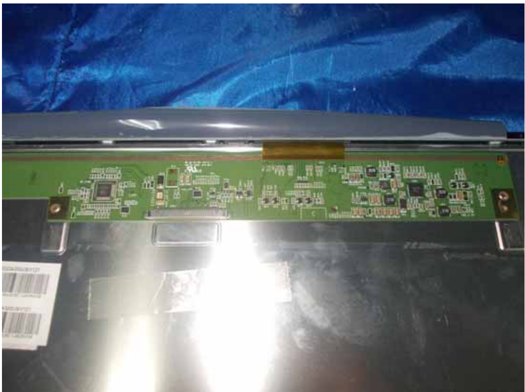
FIGURE 12 LED LCD TV (M/N: LHD23A300US) LCD PANEL CONTROL BOARD (COMPONENT SIDE)
