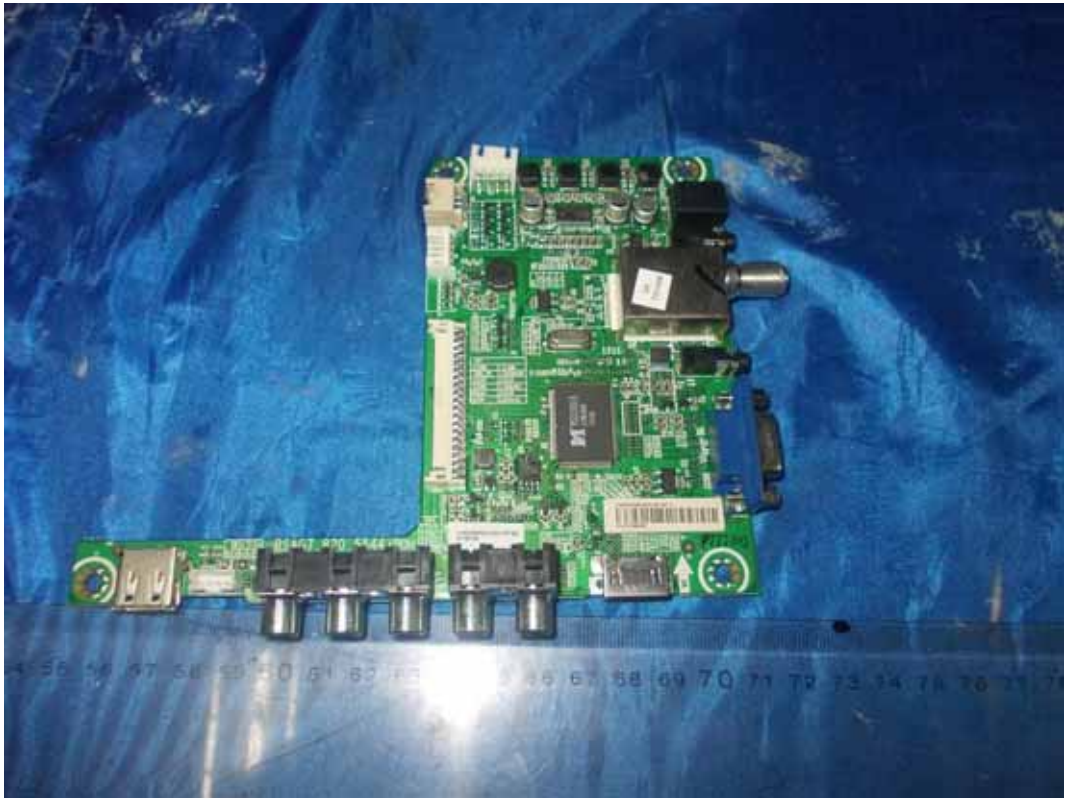
FIGURE 5 LED LCD TV (M/N: LHD23A300US) MAIN BOARD (COMPONENT SIDE)
