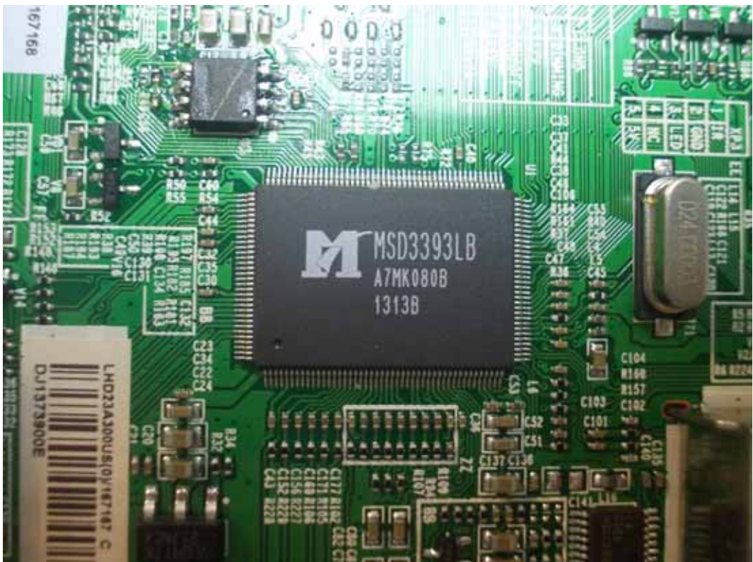
FIGURE 8 LED LCD TV (M/N: LHD23A300US) CHIP & CRYSTAL ON MAIN BOARD
