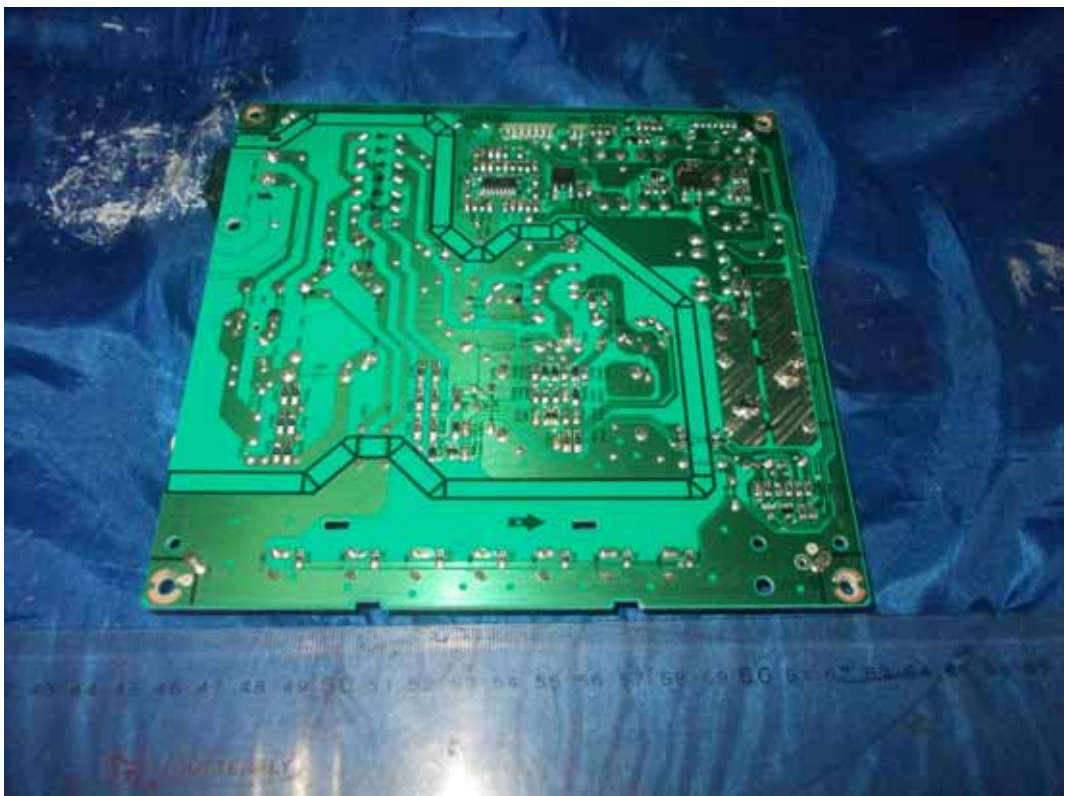
FIGURE 4 LED LCD TV (M/N: LHD23A300US) POWER BOARD (SOLDERED SIDE)
