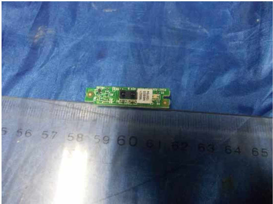
FIGURE 9 LED LCD TV (M/N: LHD23A300US) IR BOARD (COMPONENT SIDE)
