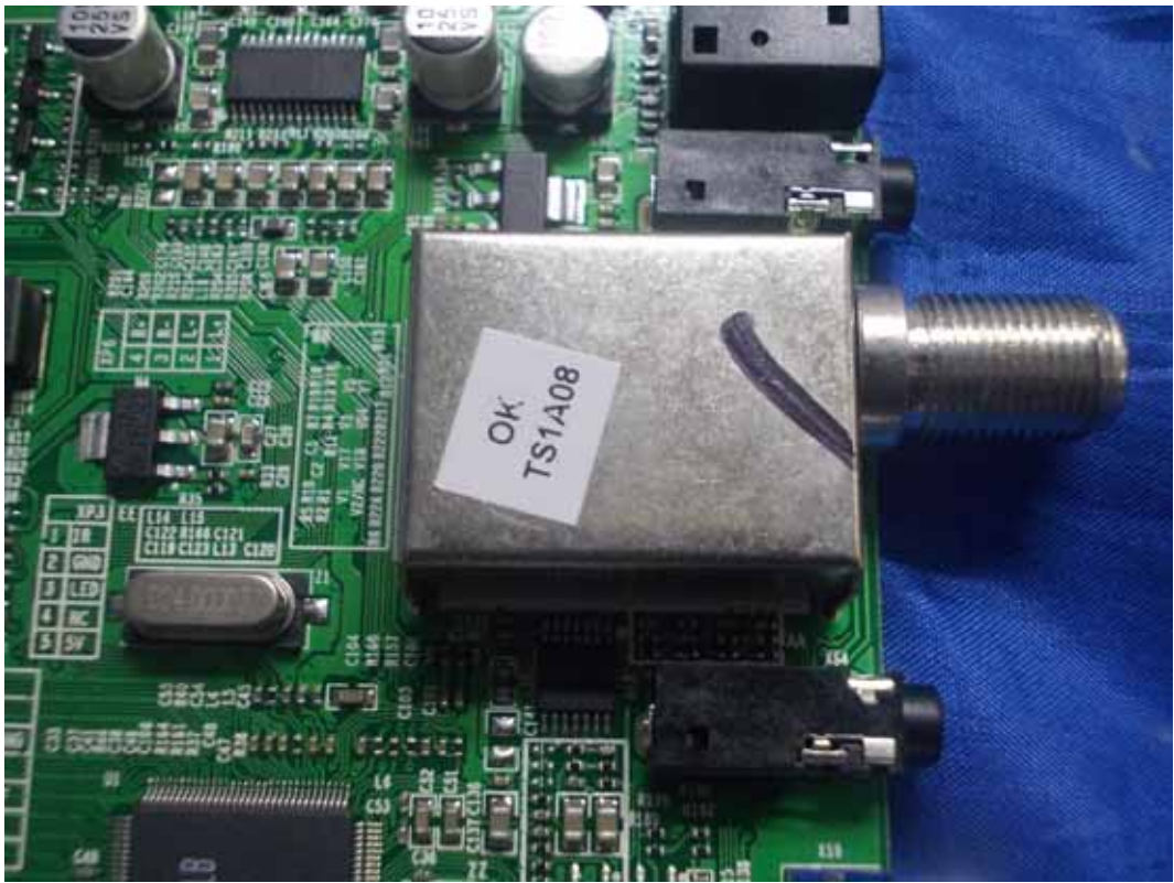
FIGURE 7 LED LCD TV (M/N: LHD23A300US) TUNER ON MAIN BOARD
