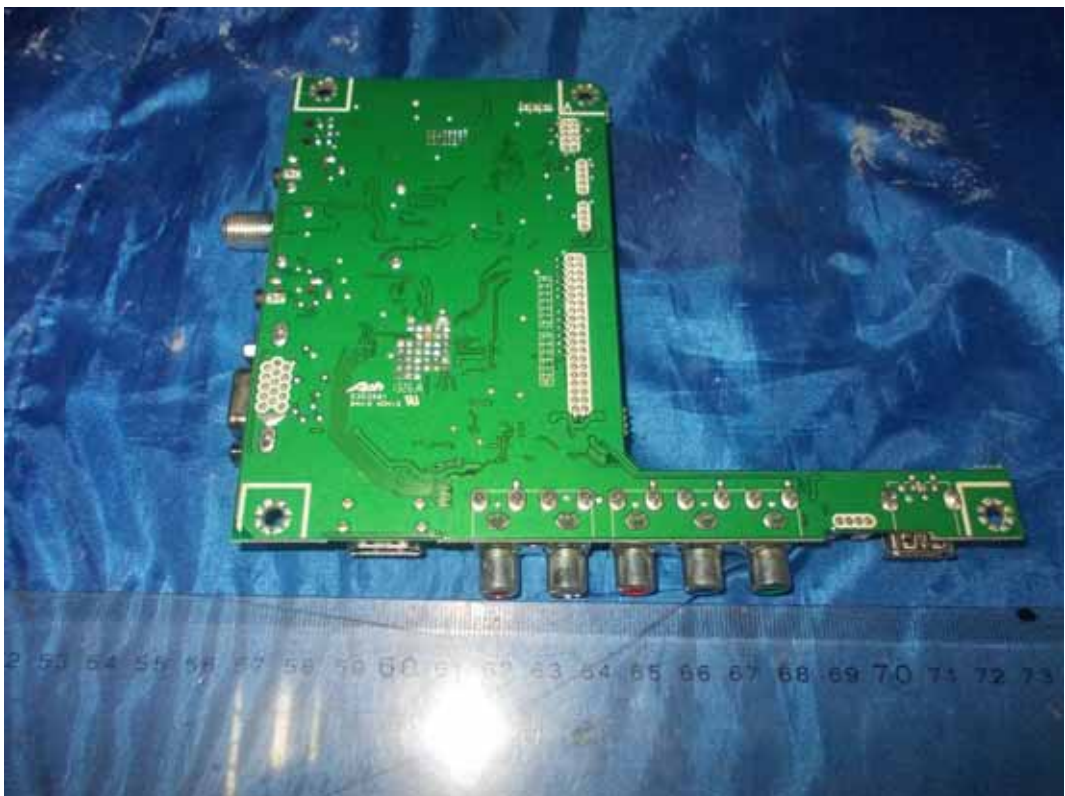
FIGURE 6 LED LCD TV (M/N: LHD23A300US) MAIN BOARD (SOLDERED SIDE)
