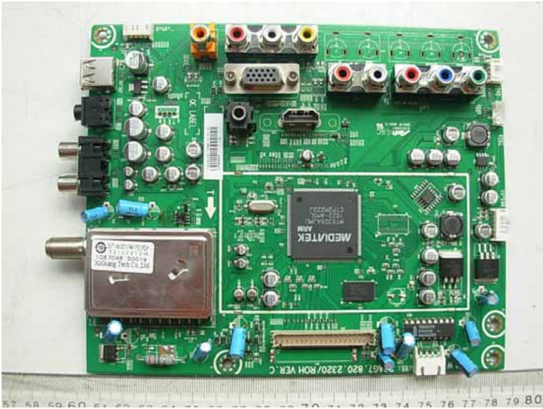
FIGURE 5 LCD TV (M/N: LEDN24K15PUS) MAIN BOARD (COMPONENT SIDE)
