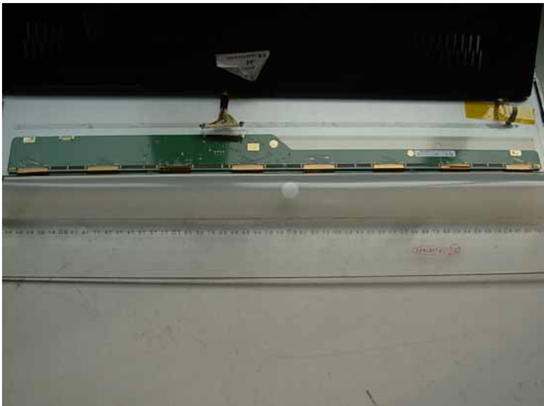
FIGURE 14 LCD TV (M/N: LEDN24K15PUS) LCD PANEL CONTROL BOARD (SOLDERED SIDE)
