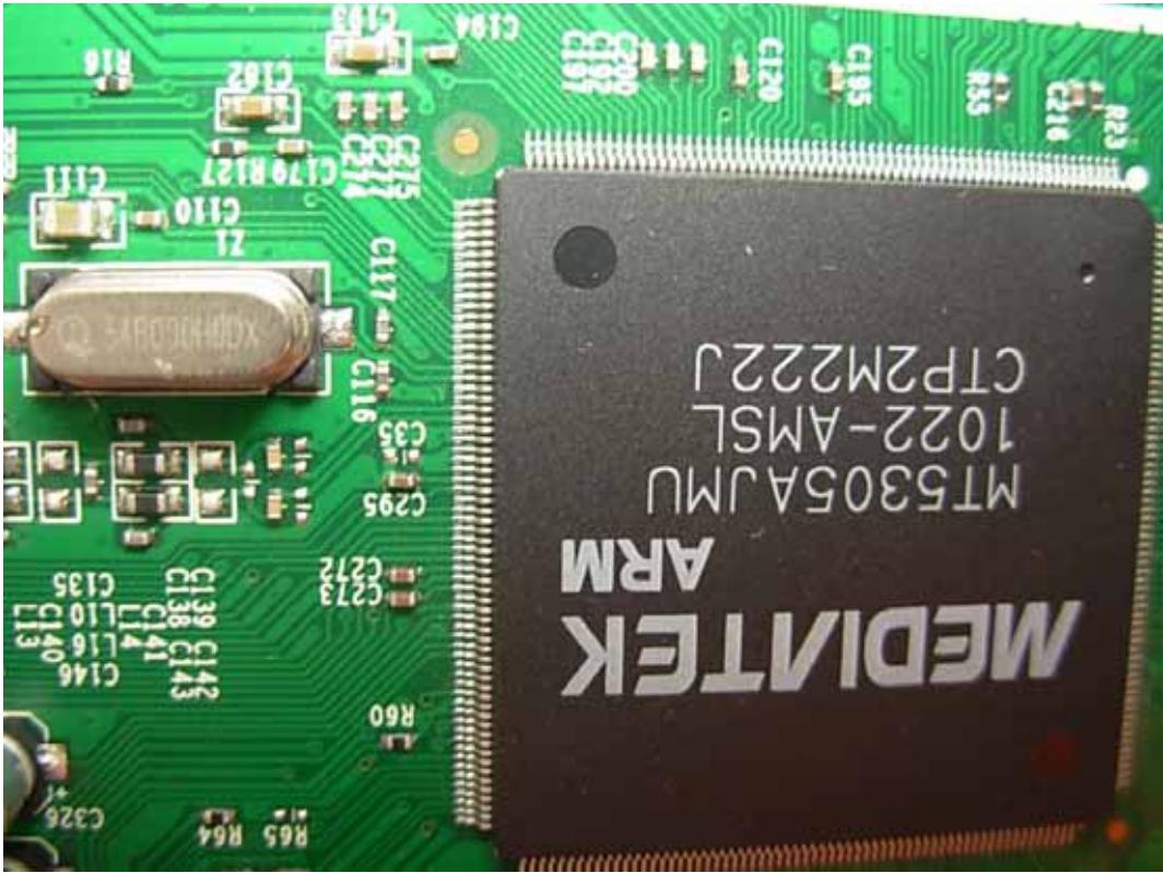
FIGURE 7 LCD TV (M/N: LEDN24K15PUS) CRYSTAL & CHIP ON MAIN BOARD
