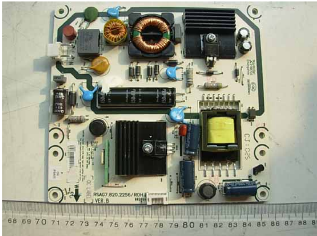
FIGURE 3 LCD TV (M/N: LEDN24K15PUS) POWER BOARD (COMPONENT SIDE)
