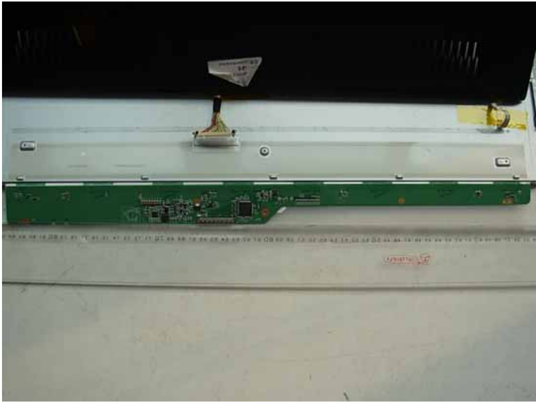
FIGURE 13 LCD TV (M/N: LEDN24K15PUS) LCD PANEL CONTROL BOARD (COMPONENT SIDE)
