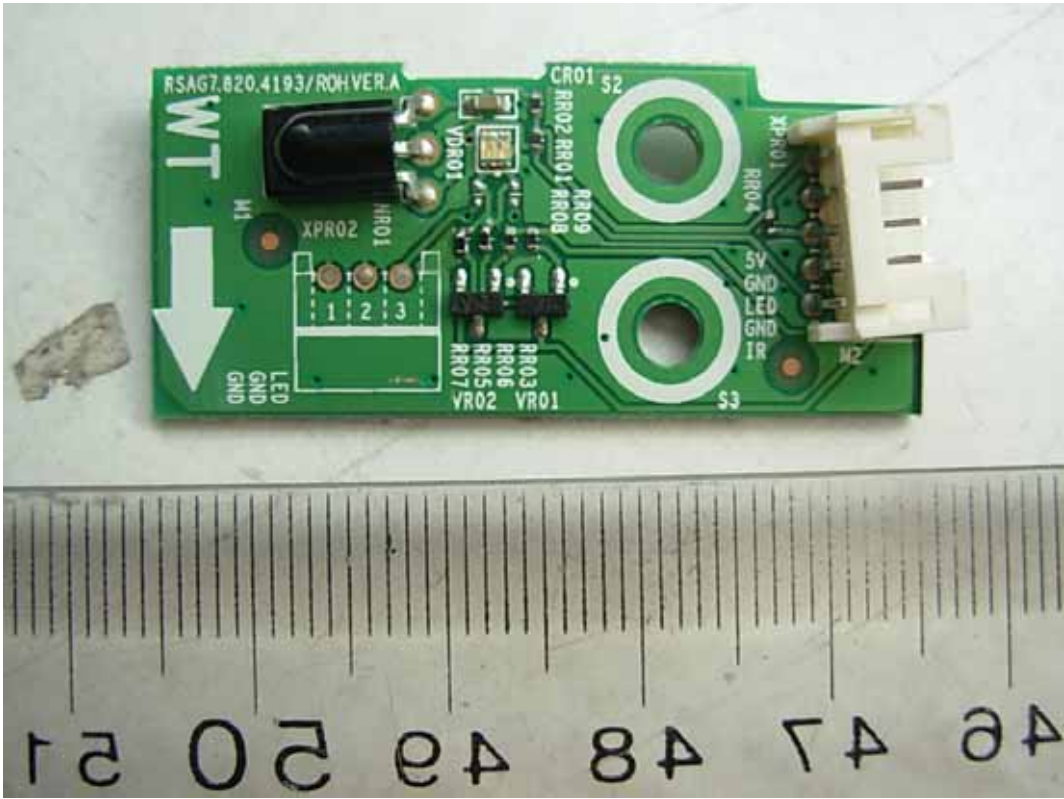
FIGURE 9 LCD TV (M/N: LEDN24K15PUS) IR BOARD (COMPONENT SIDE)
