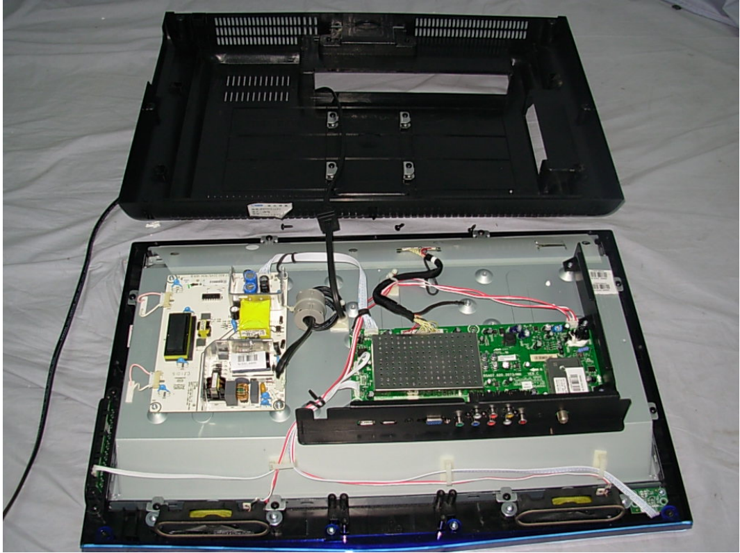
FIGURE 1 LCD TV (M/N: LTDN24V86NUS) COVER REMOVED
