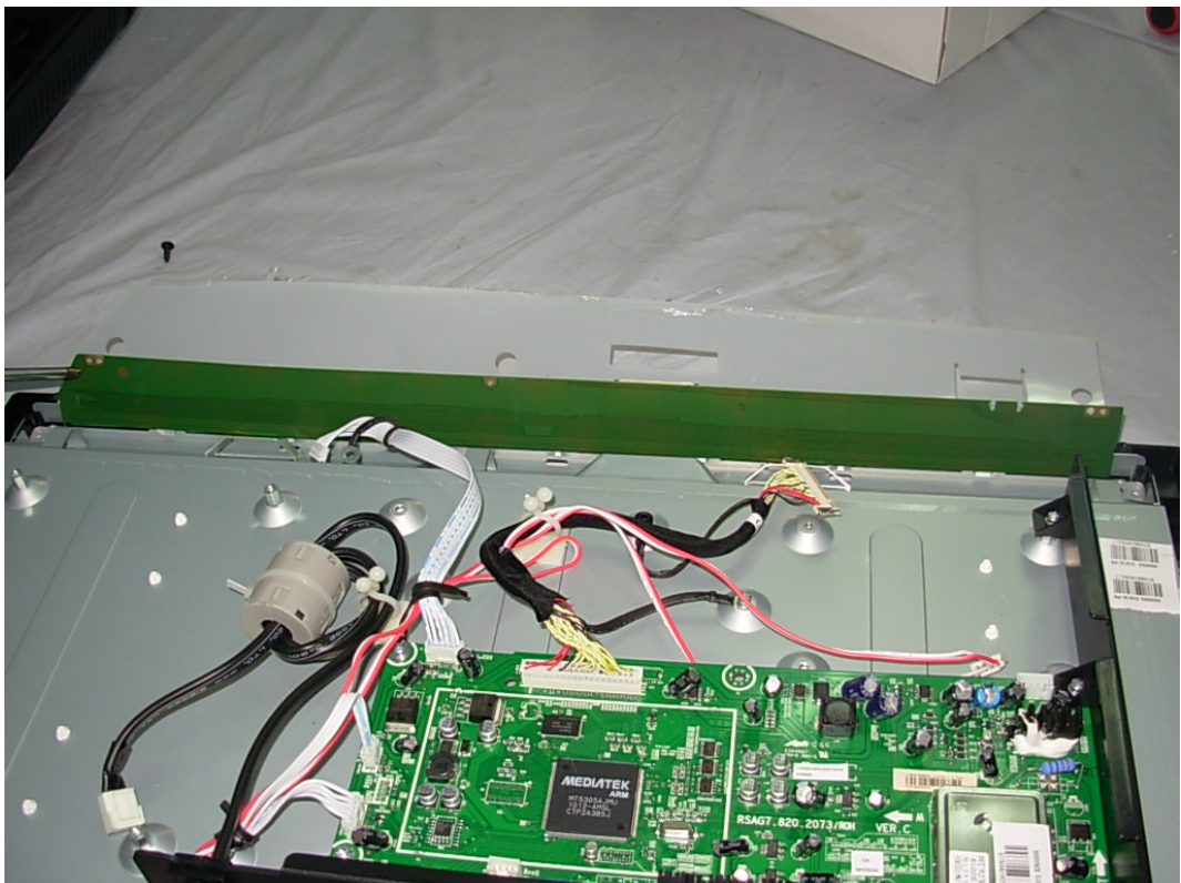
FIGURE 12 LCD TV (M/N: LTDN24V86NUS) LCD PANEL MAIN BOARD (SOLDERED SIDE)
