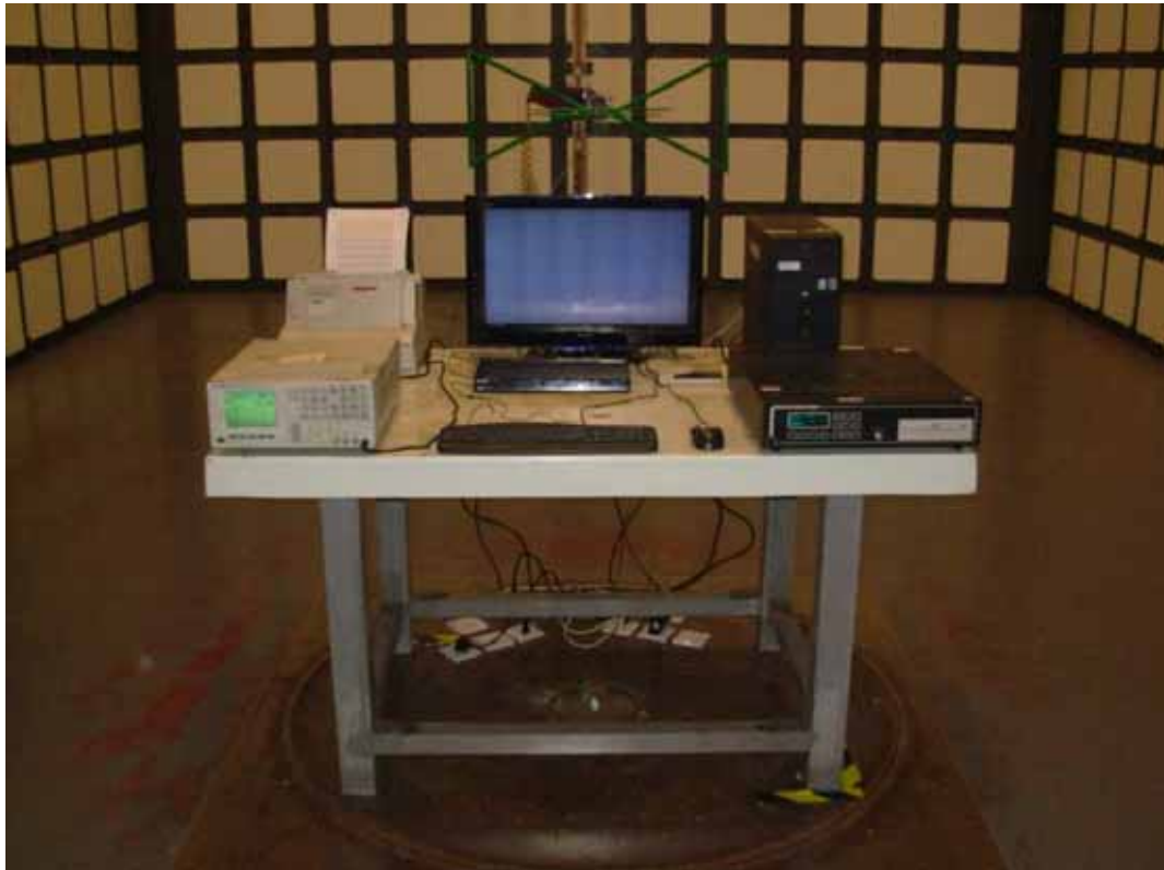
FRONT VIEW OF RADIATED EMISSION TEST
