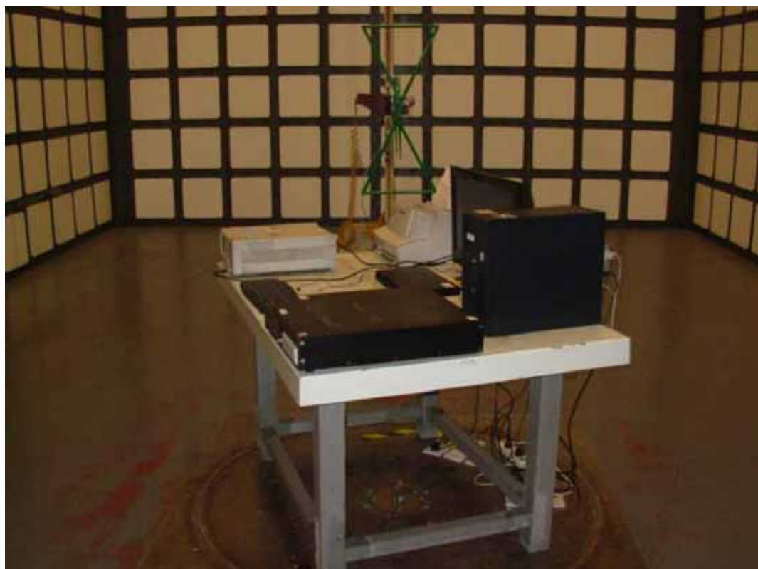
SETUP WITH MAXIMUM DETECTED EMISSION AT VERTICAL POLARIZATION (D-SUB 1024*768@60Hz)
