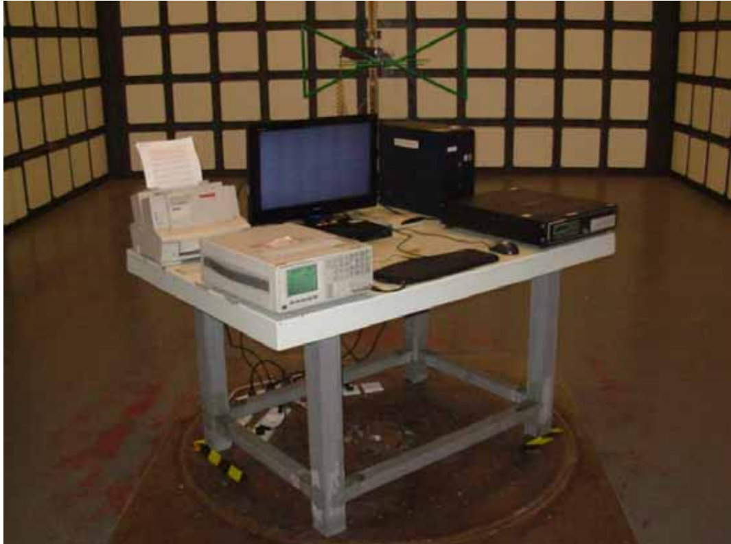
SETUP WITH MAXIMUM DETECTED EMISSION AT HORIZONTAL POLARIZATION (D-SUB 1024*768@60Hz)
