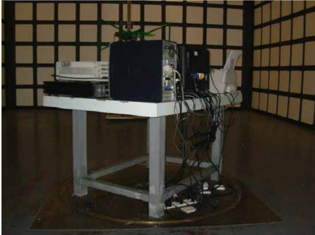
SETUP WITH MAXIMUM DETECTED EMISSION AT HORIZONTAL POLARIZATION (HDMI 640*480@60Hz)
