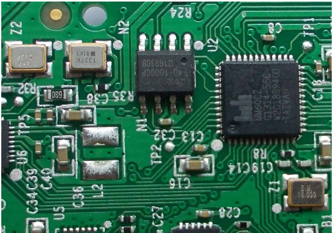
FIGURE 7 PULSE REMOTE CONTROL (M/N: ERF6B11) CHIP & CRYSTAL ON MAIN BOARD
