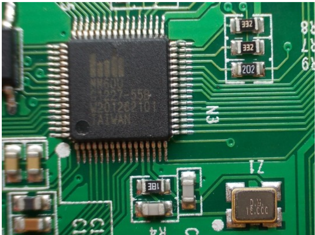
FIGURE 8 HISENSE PULSE WITH GOOGLE TV REMOTE CONTROL (M/N: ERF6B10) CHIP & CRYSTAL #1 ON MAIN BOARD
