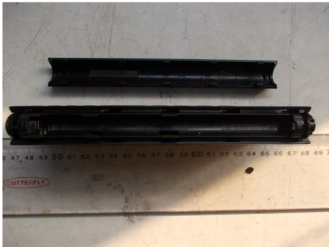
FIGURE 3 HISENSE PULSE WITH GOOGLE TV REMOTE CONTROL (M/N: ERF6B10) BATTERY COVER REMOVED
