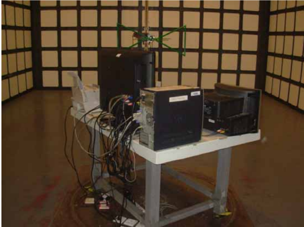
SETUP WITH MAXIMUM DETECTED EMISSION AT HORIZONTAL POLARIZATION (D-SUB 1360*768@60Hz)
