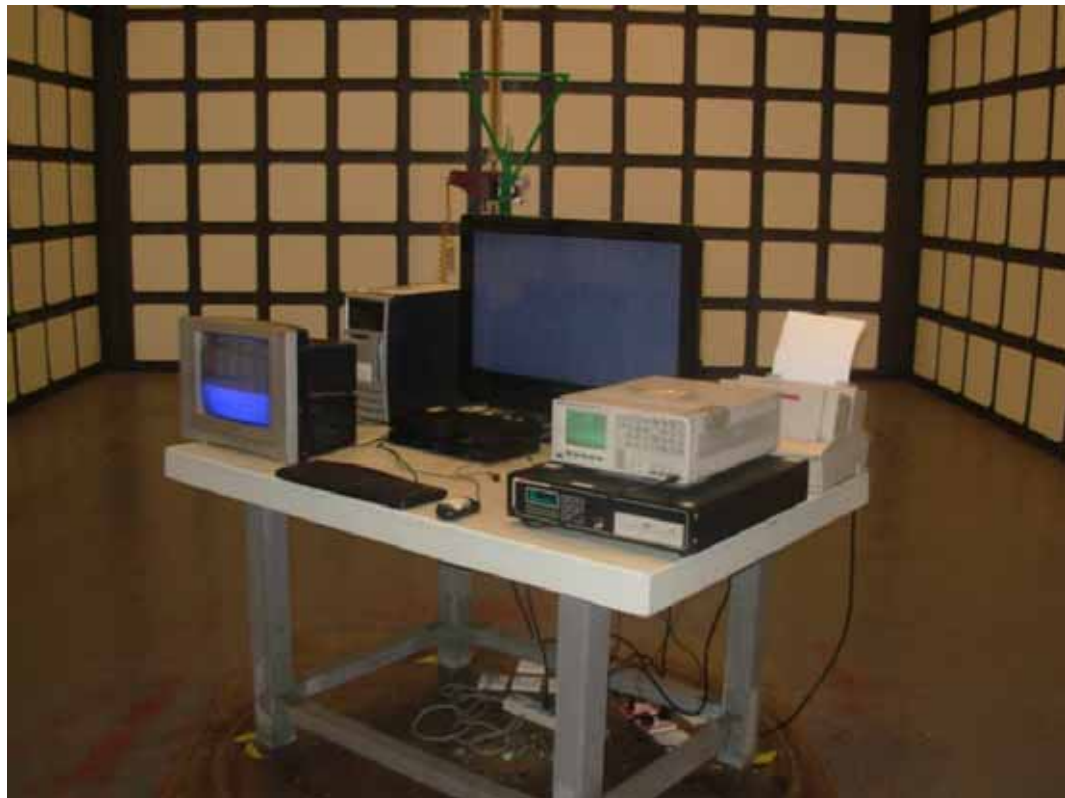
SETUP WITH MAXIMUM DETECTED EMISSION AT VERTICAL POLARIZATION (D-SUB 1360*768@60Hz)
