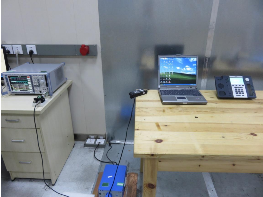
FCC RADIATED EMISSION TEST SETUP BELOW 1GHZ
