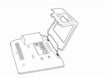
B. Press the other side joints into the slot according to the direction of the arrow
