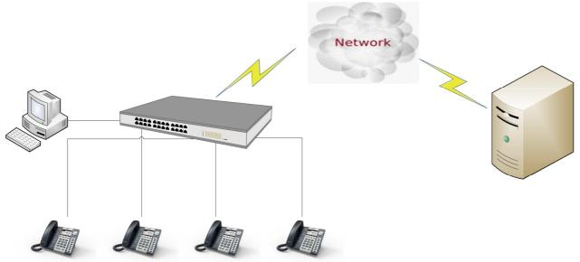
Connect LAN port to PC with Ethernet cable, or connect A40/A41(W) to a switch/router which is in the same network as your PC. It uses DHCP mode by default, and you can review its current IP address
