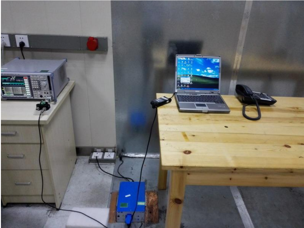
FCC RADIATED EMISSION TEST SETUP BELOW 1GHZ
