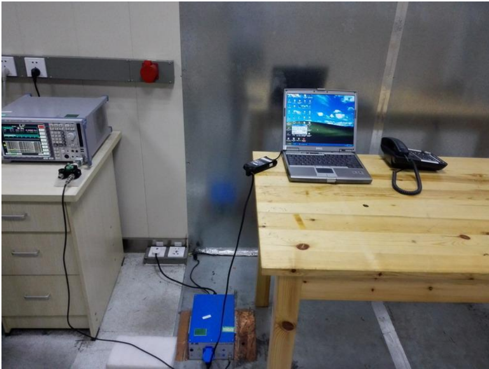
FCC RADIATED EMISSION TEST SETUP BELOW 1GHZ
