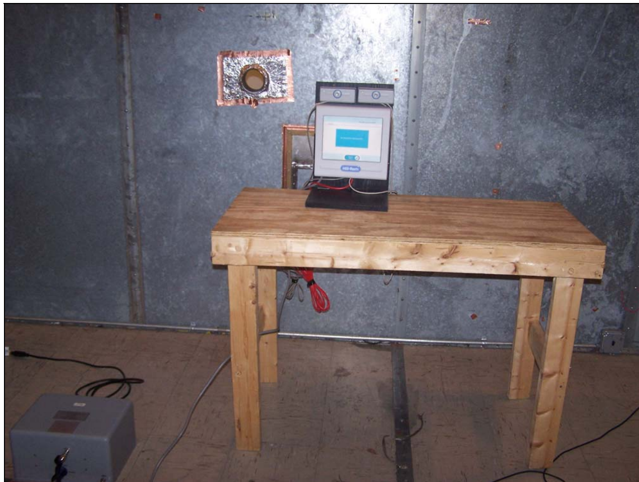
Photograph 2. Conducted Emissions, Test Setup
