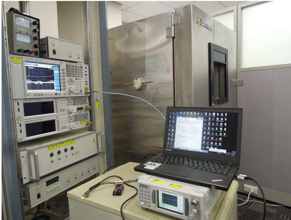
Photograph 8: Set-up for Conducted testing
