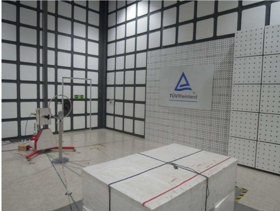
Photograph 6: Set-up for Spurious Emissions (Back View 4)
