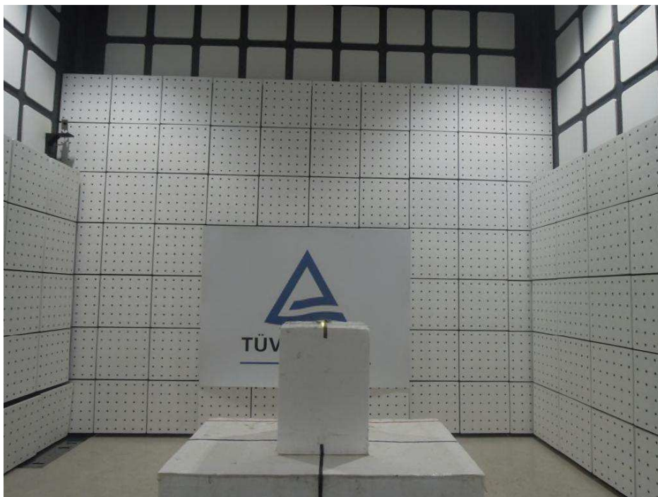
Photograph 2: Set-up for Spurious Emissions (Front View 2)
