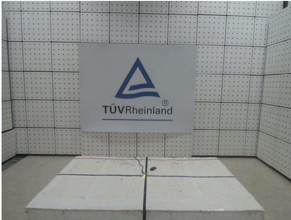
Photograph 2: Set-up for Spurious Emissions (Front View 2)
