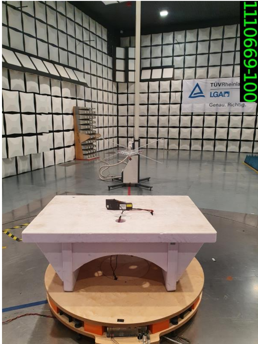
Test Setup: Radiated Measurements (30 MHz - 1 GHz)
