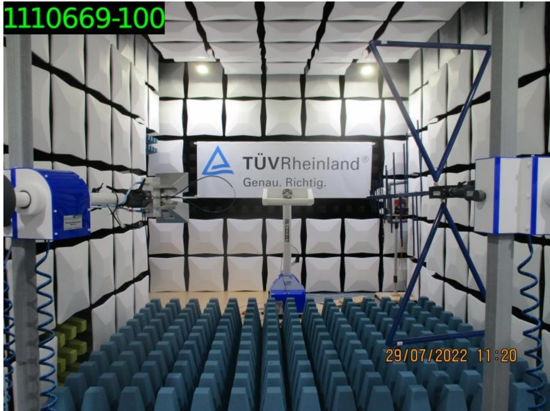
Test Setup: Radiated Measurements (1 GHz to 26.5 GHz)
