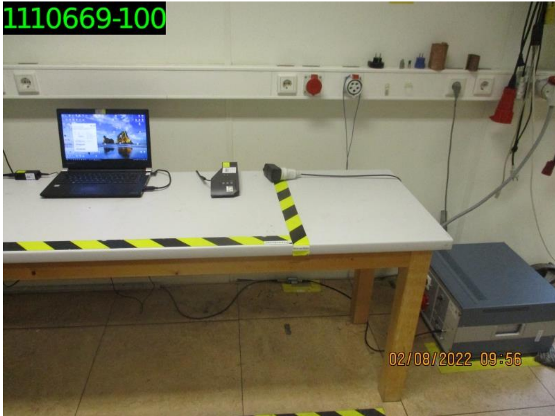
Test Setup: Conducted Emission Measurements
