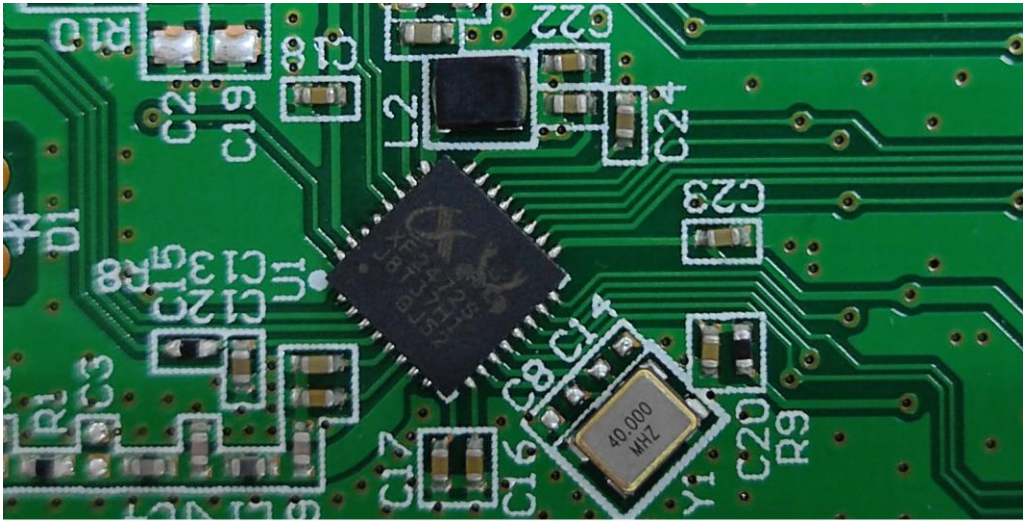
PCB with IC: RTL8752CRF
