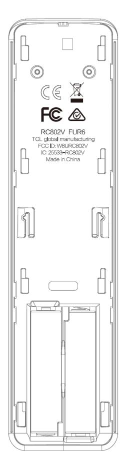
Label location is within the battery compartment
