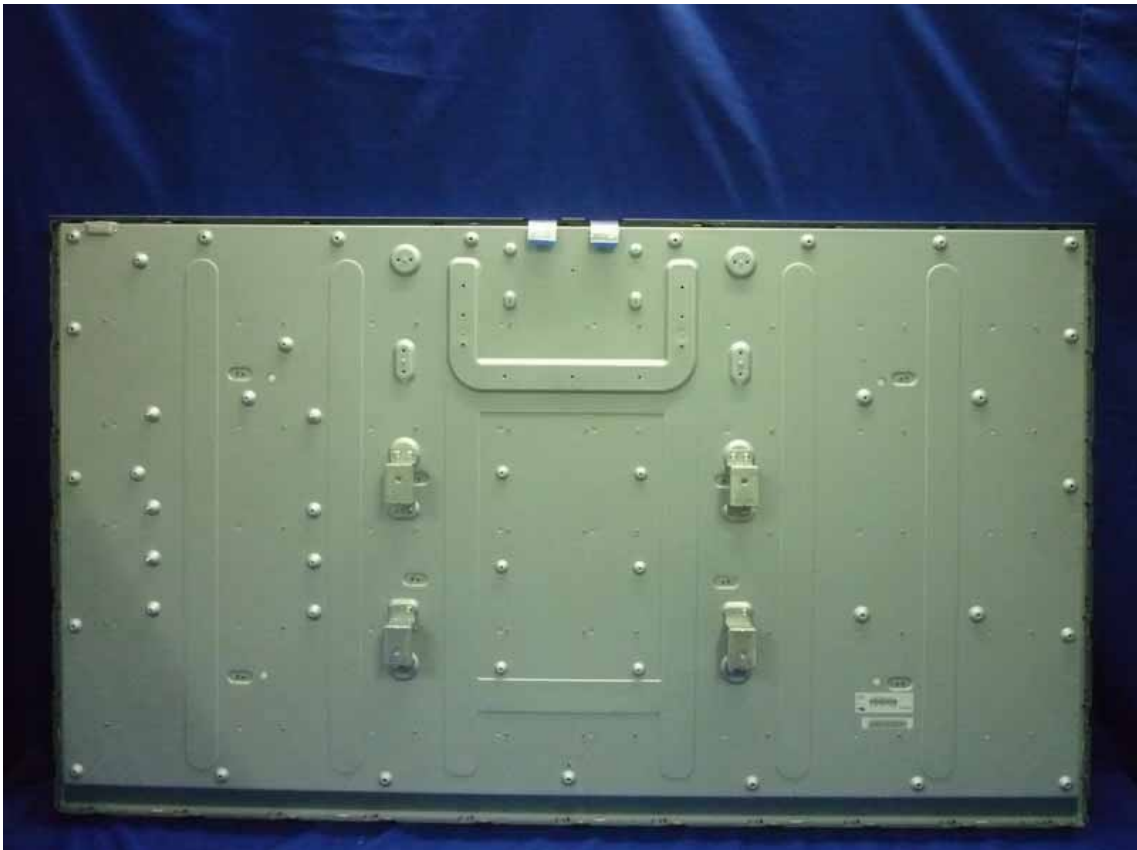
Figure 14 Backside of the LCD Panel
