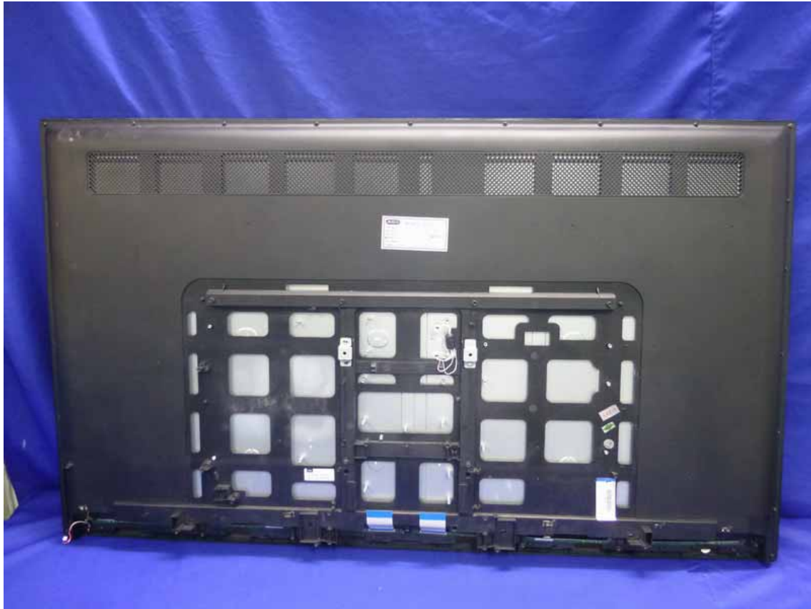
Figure 15 Backside of the LCD Panel
