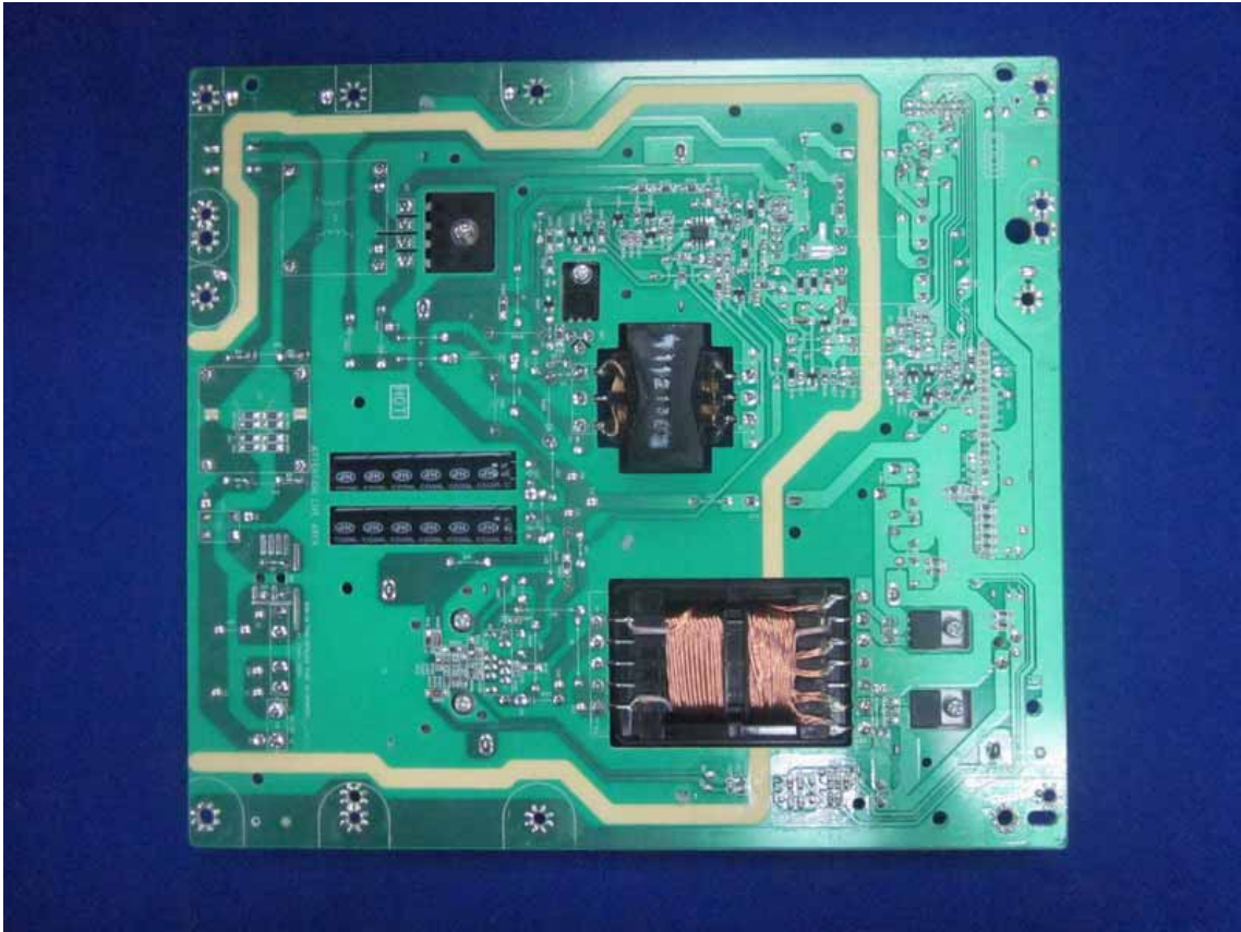
Figure 20 Backside of the Power Board
