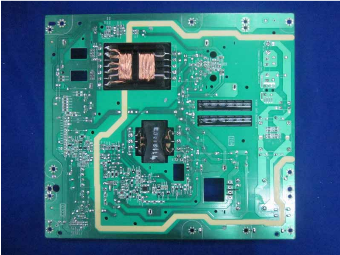
Figure 22 Backside of the Power Board
