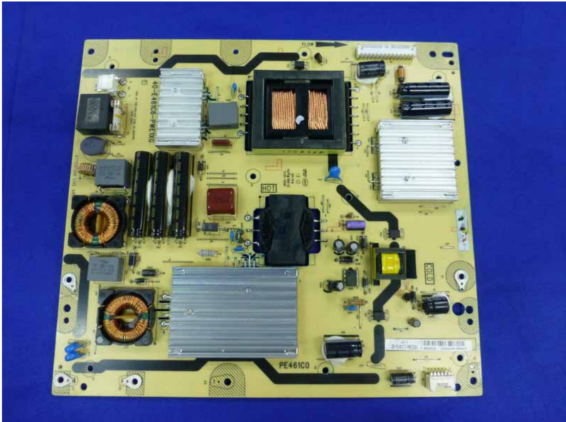
Figure 19 Frontside of the Power Board
