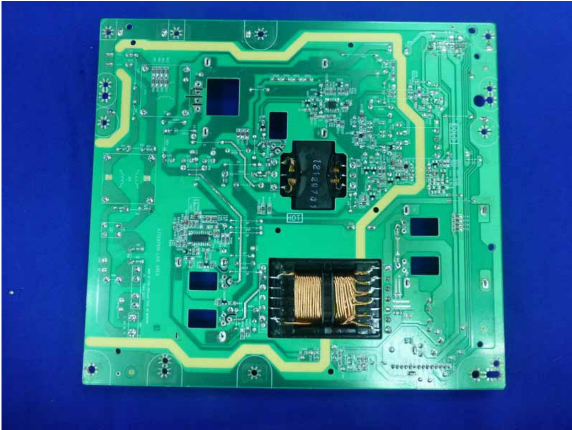
Figure 21 Frontside of the Power Board
