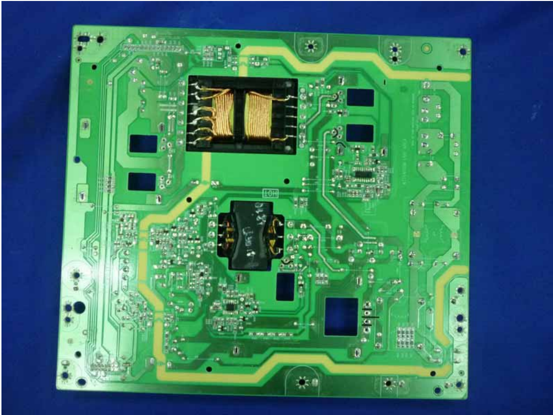
Figure 19 Backside of the Power Board
