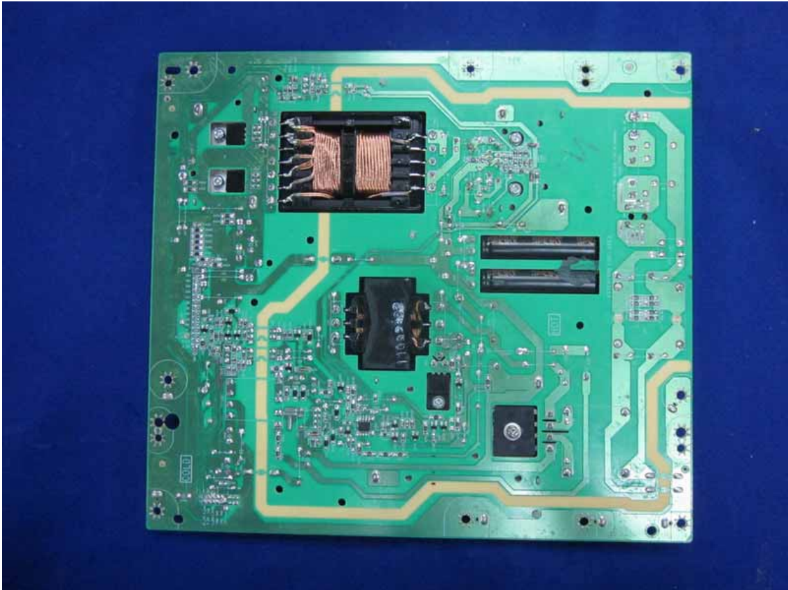
Figure 16 Backside of the Power Board
