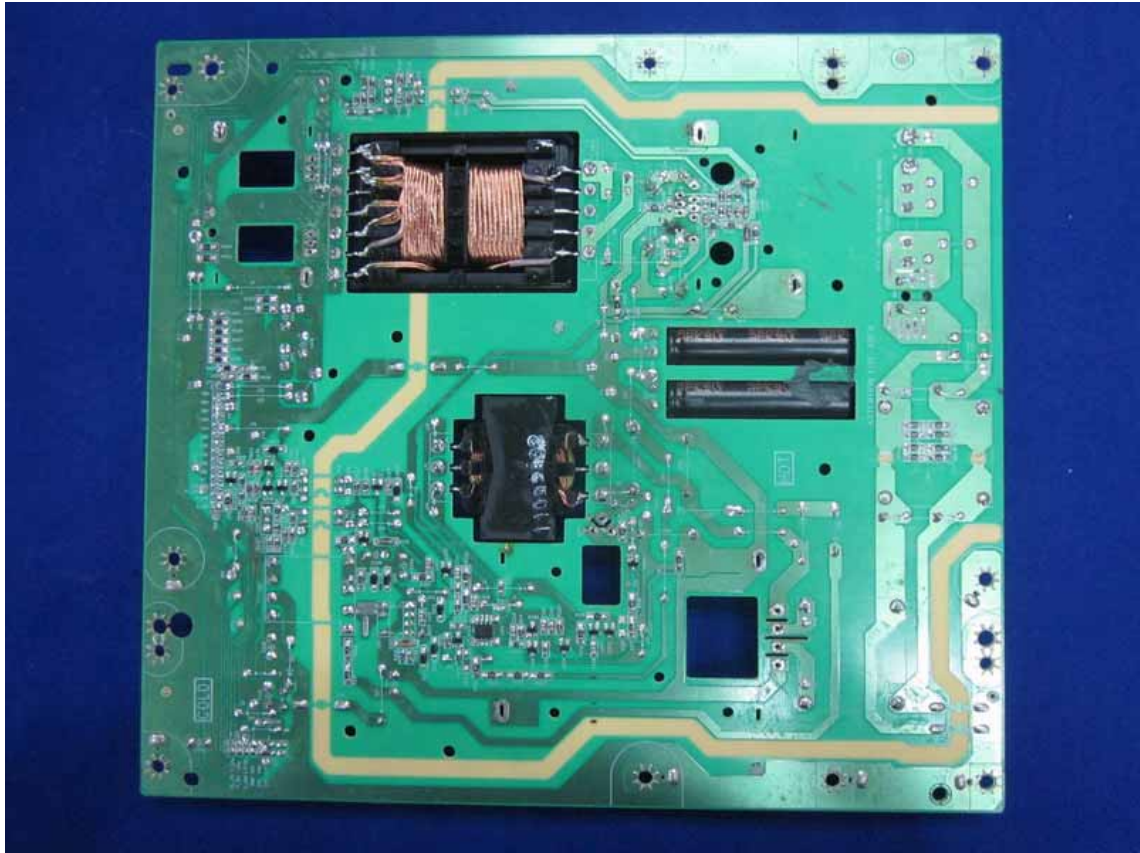
Figure 18 Backside of the Power Board
