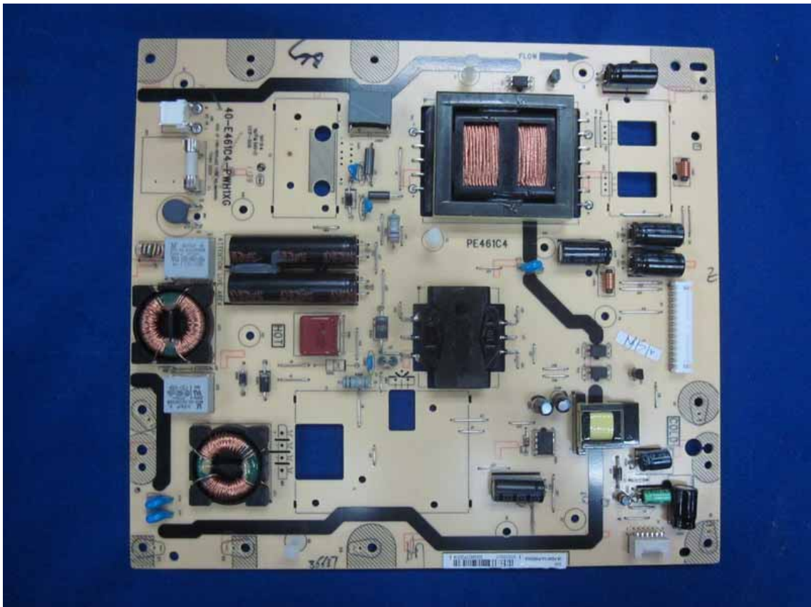
Figure 17 Frontside of the Power Board
