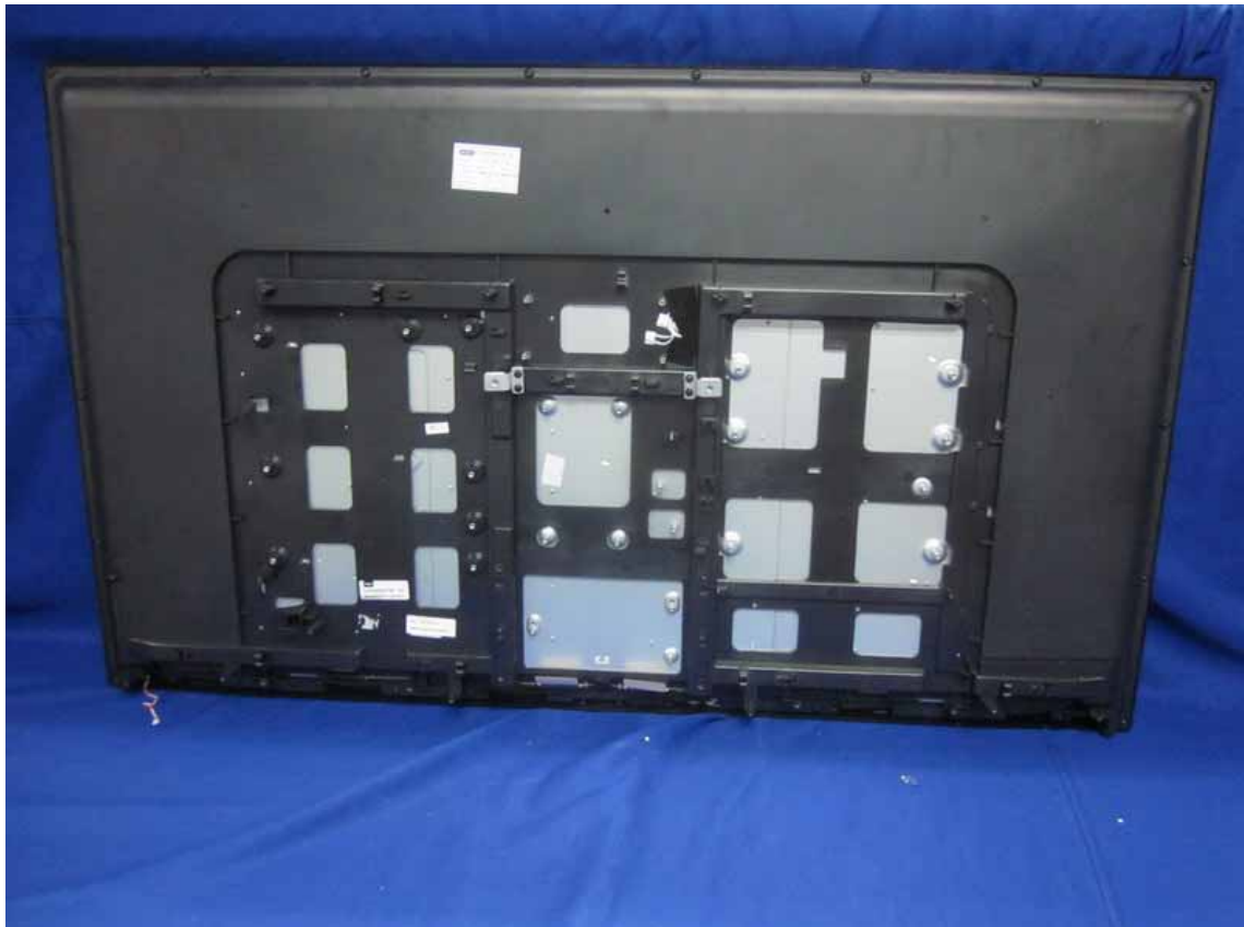
Figure 11 Backside of the LCD Panel
