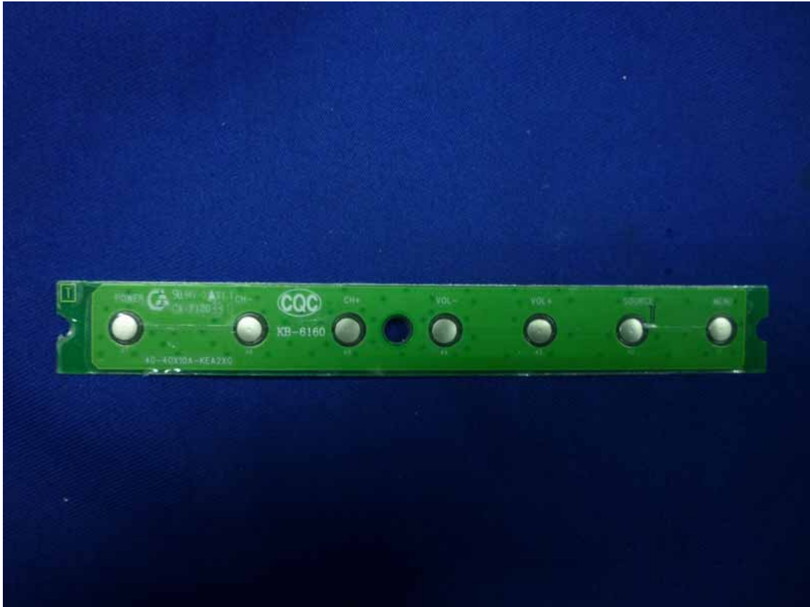
Figure 23 Frontside of the Control Board
