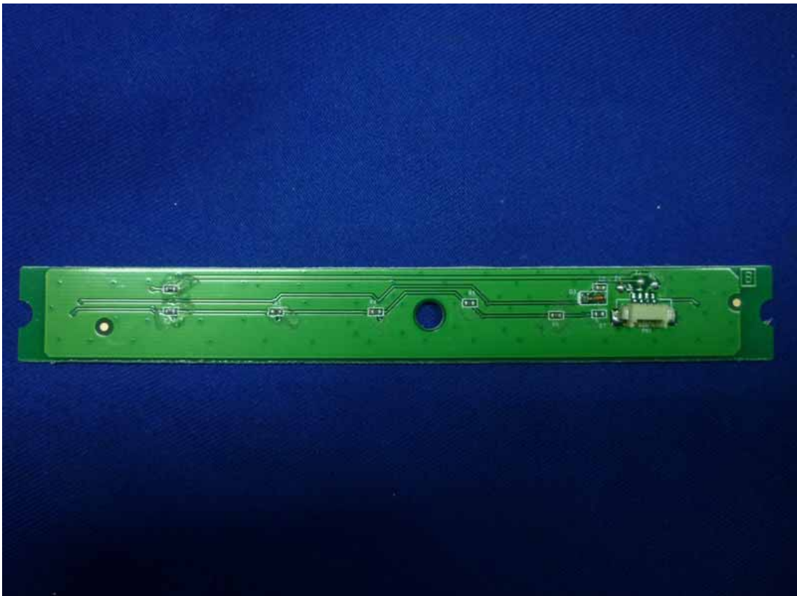
Figure 24 Backside of the Control Board
