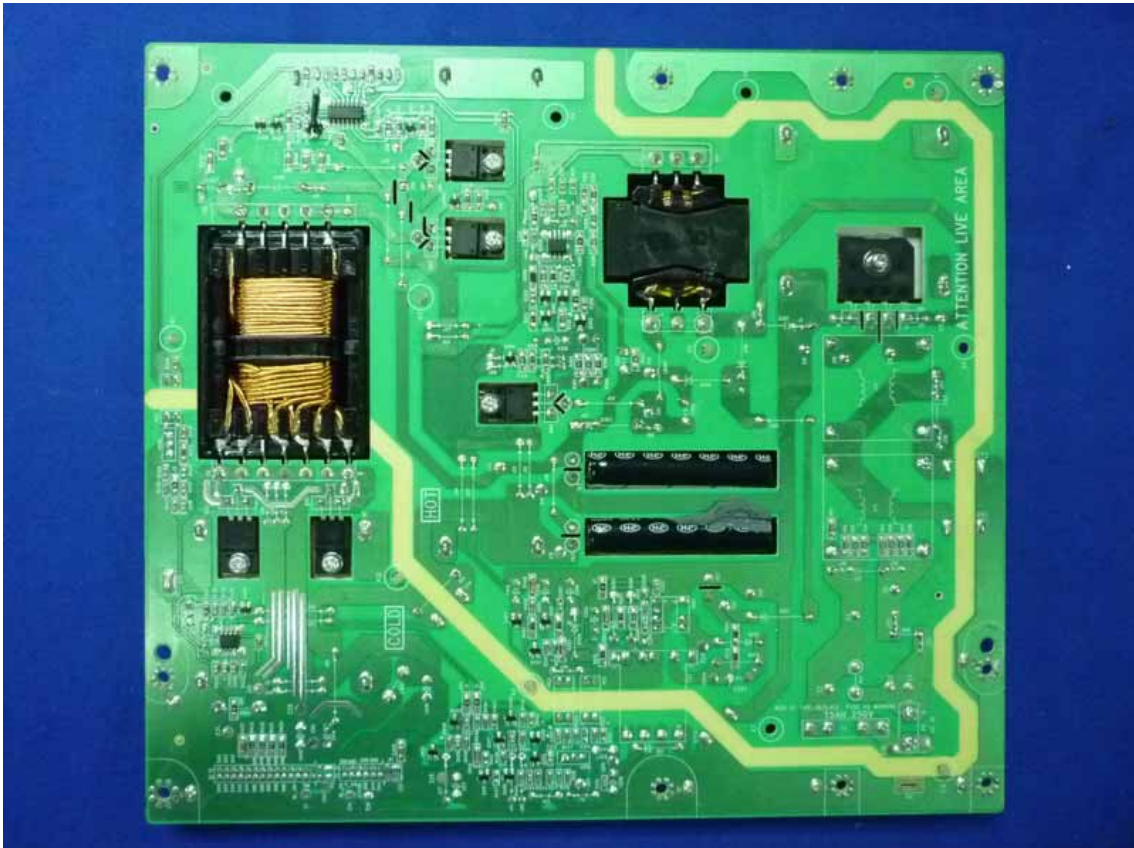
Figure 16 Backside of the Power Board
