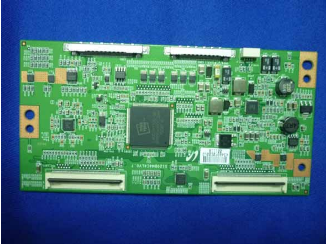
Figure 36 Backside of the Connect Board
