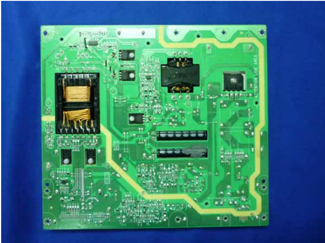
Figure 38 Backside of the Power Board
