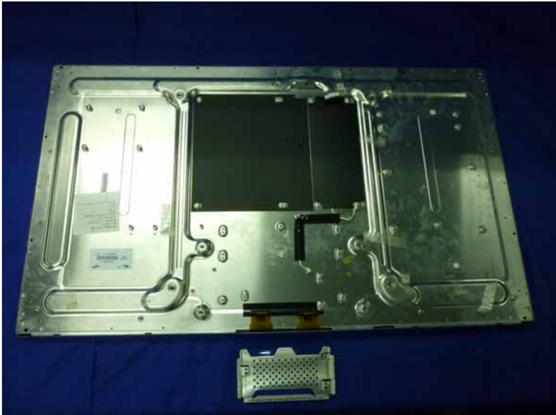
Figure 32 Backside of the LCD Panel
