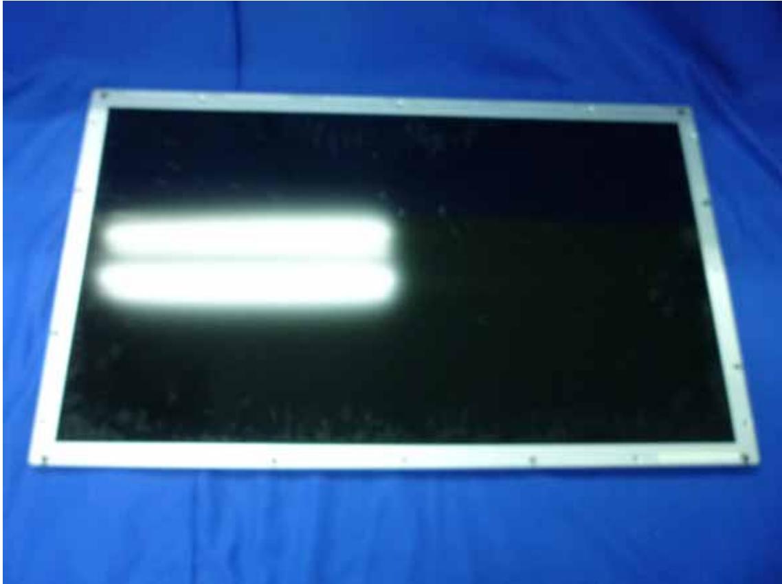
Figure 32 Backside of the LCD Panel
