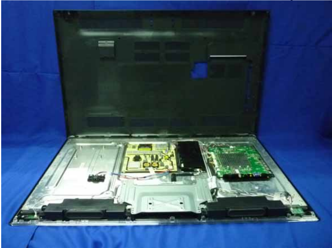
Figure 30 Inside Configuration of the EUT
