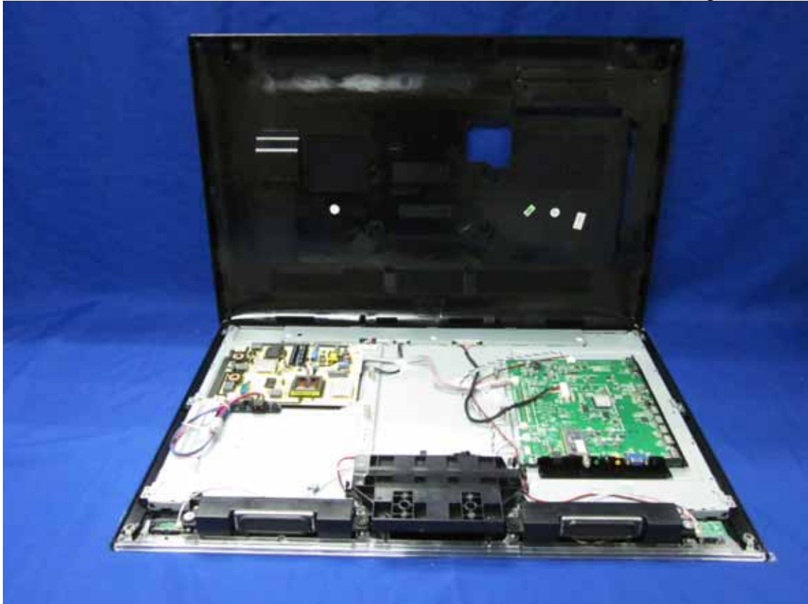
Figure 8 Inside Configuration of the EUT
