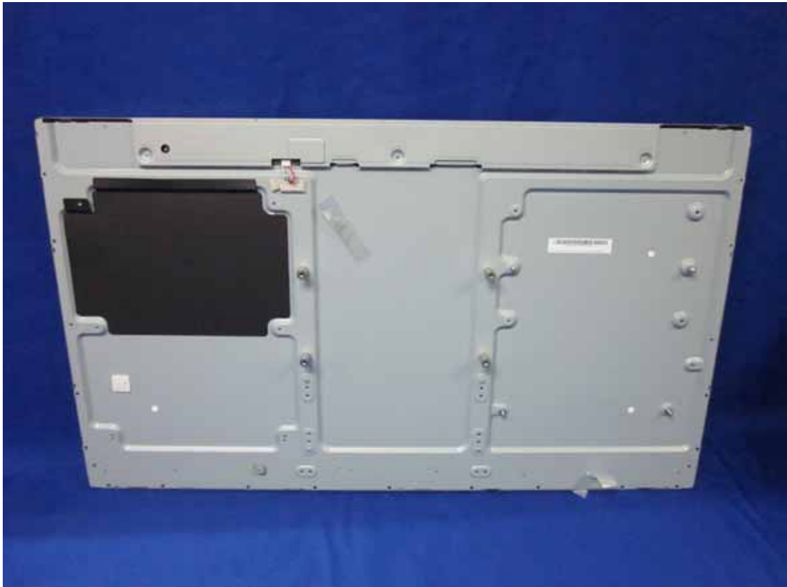
Figure 10 Backside of the LCD Panel
