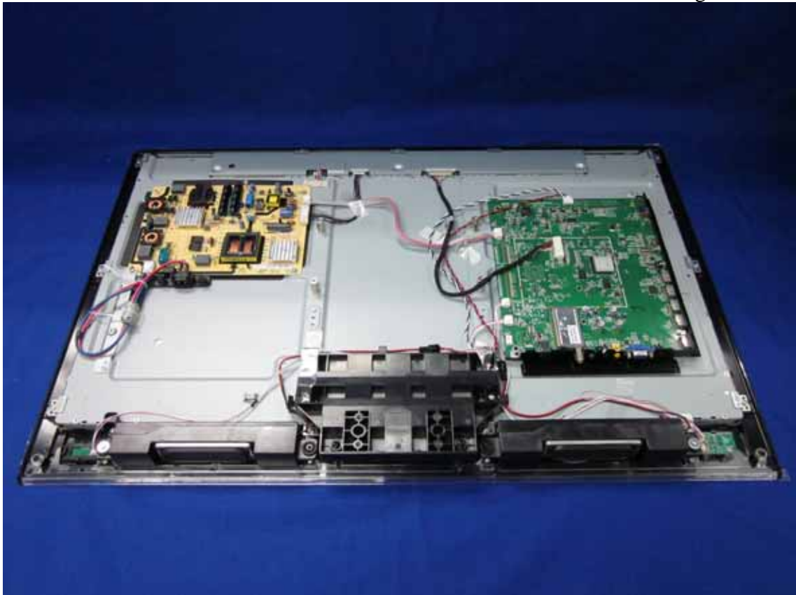
Figure 8 Inside Configuration of the EUT
