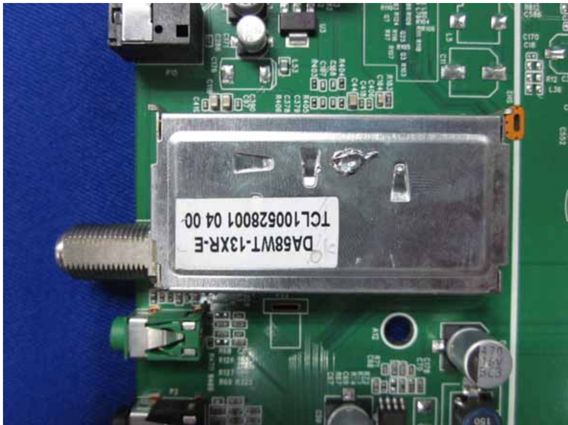
Figure 12 Tuner of the EUT
