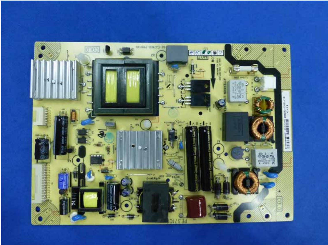
Figure 18 Frontside of the Power Board
