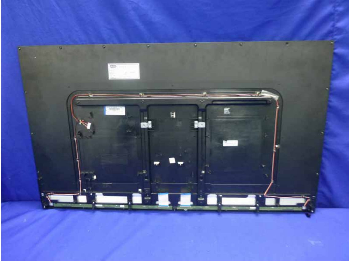
Figure 12 Backside of the LCD Panel
