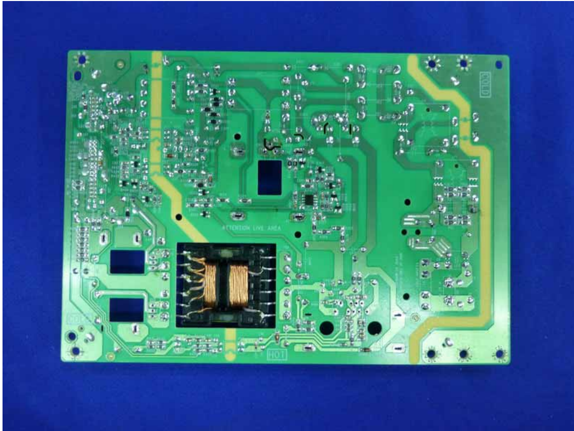
Figure 21 Frontside of the Power Board
