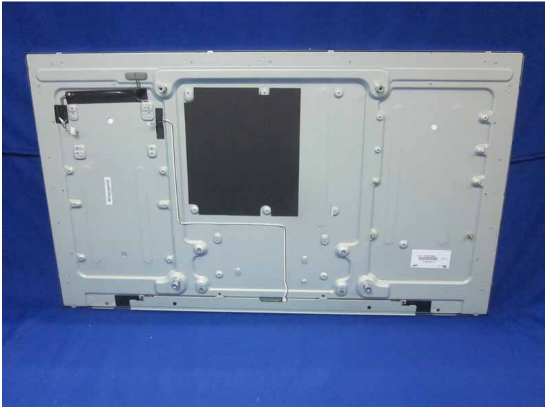
Figure 12 Backside of the LCD Panel
