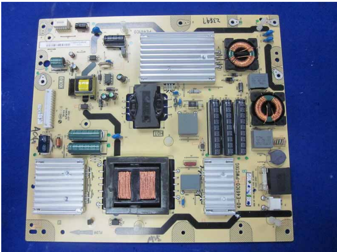
Figure 18 Frontside of the Power Board
