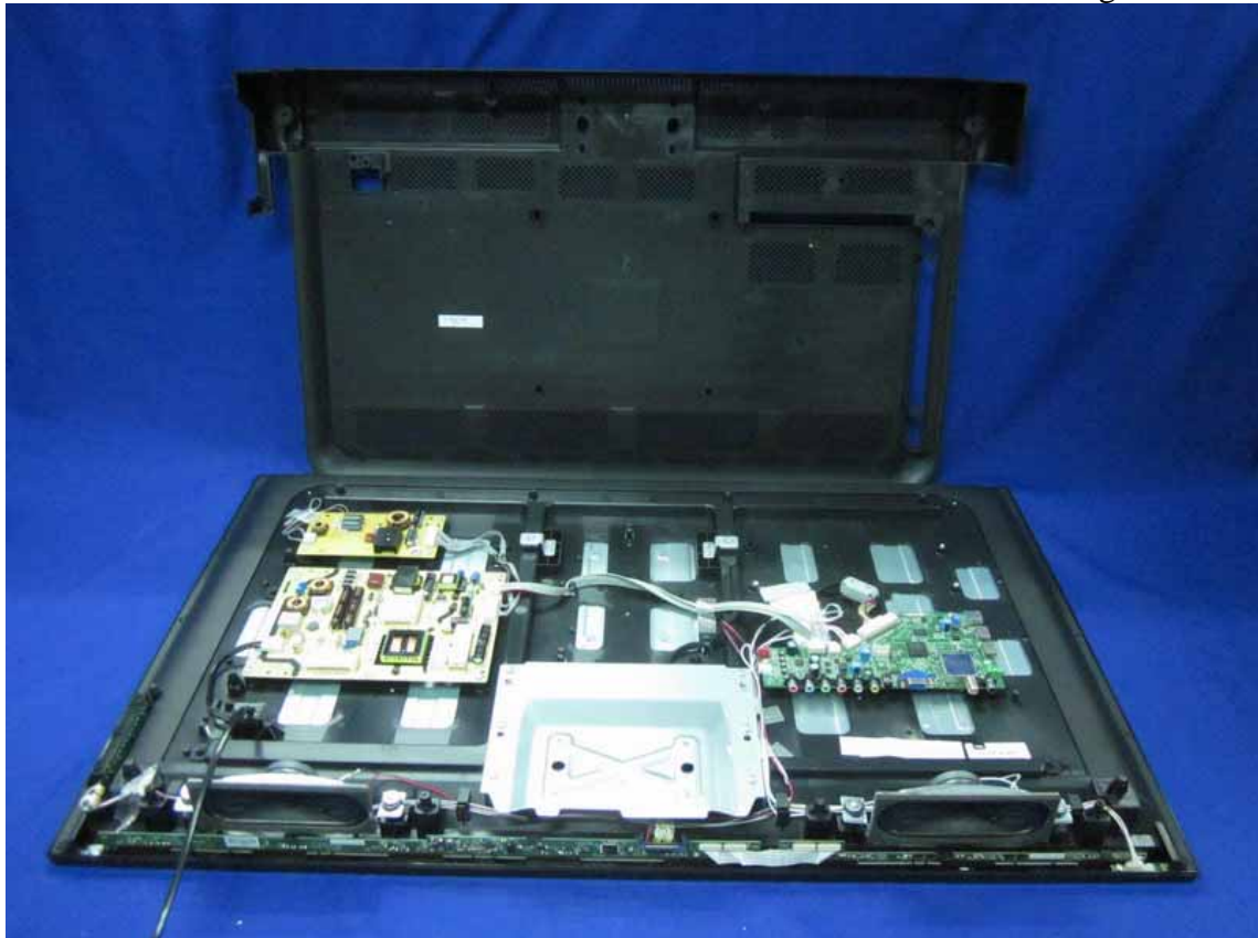
Figure 8 Inside Configuration of the EUT
