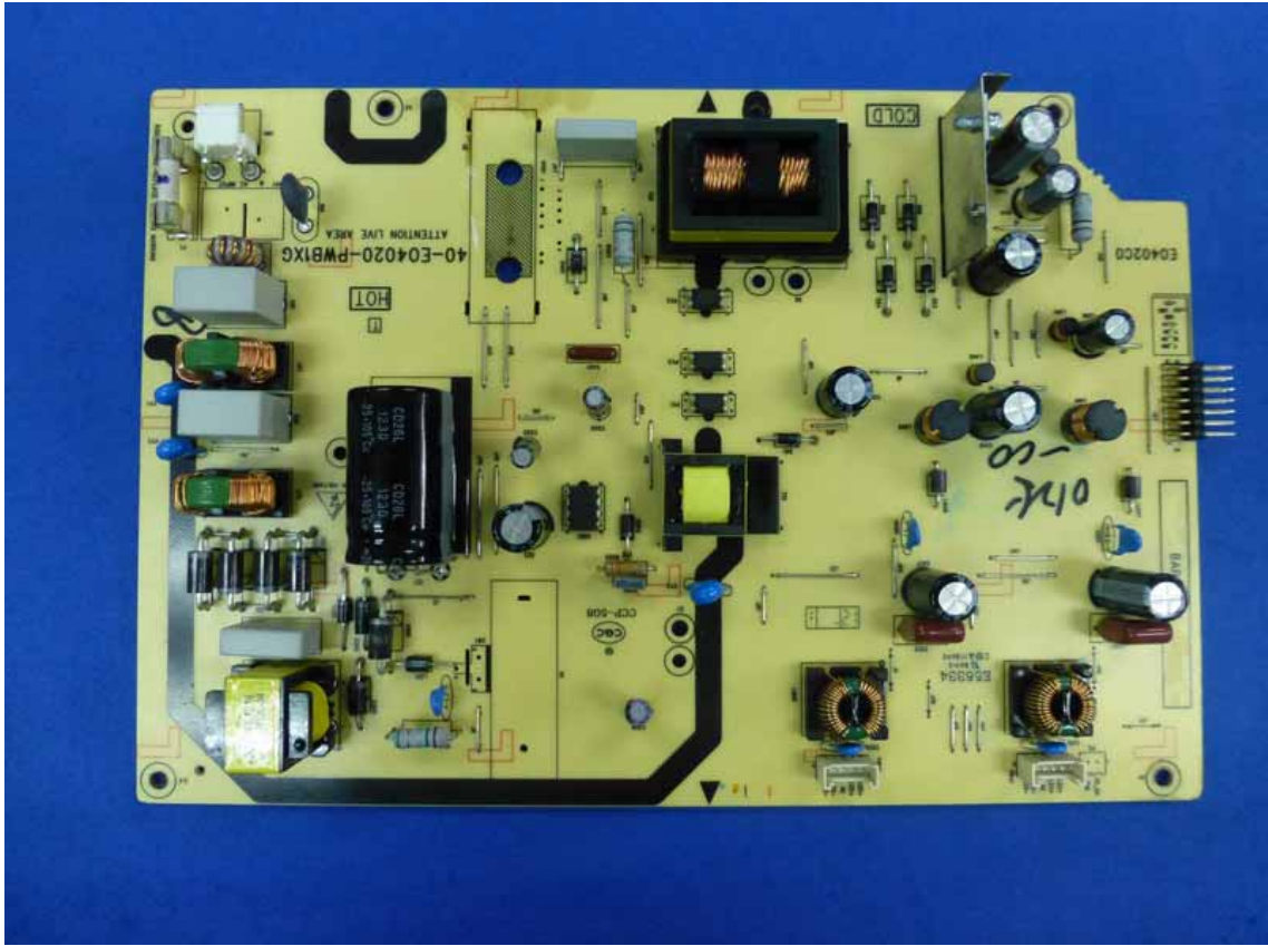
Figure 18 Frontside of the Power Board
