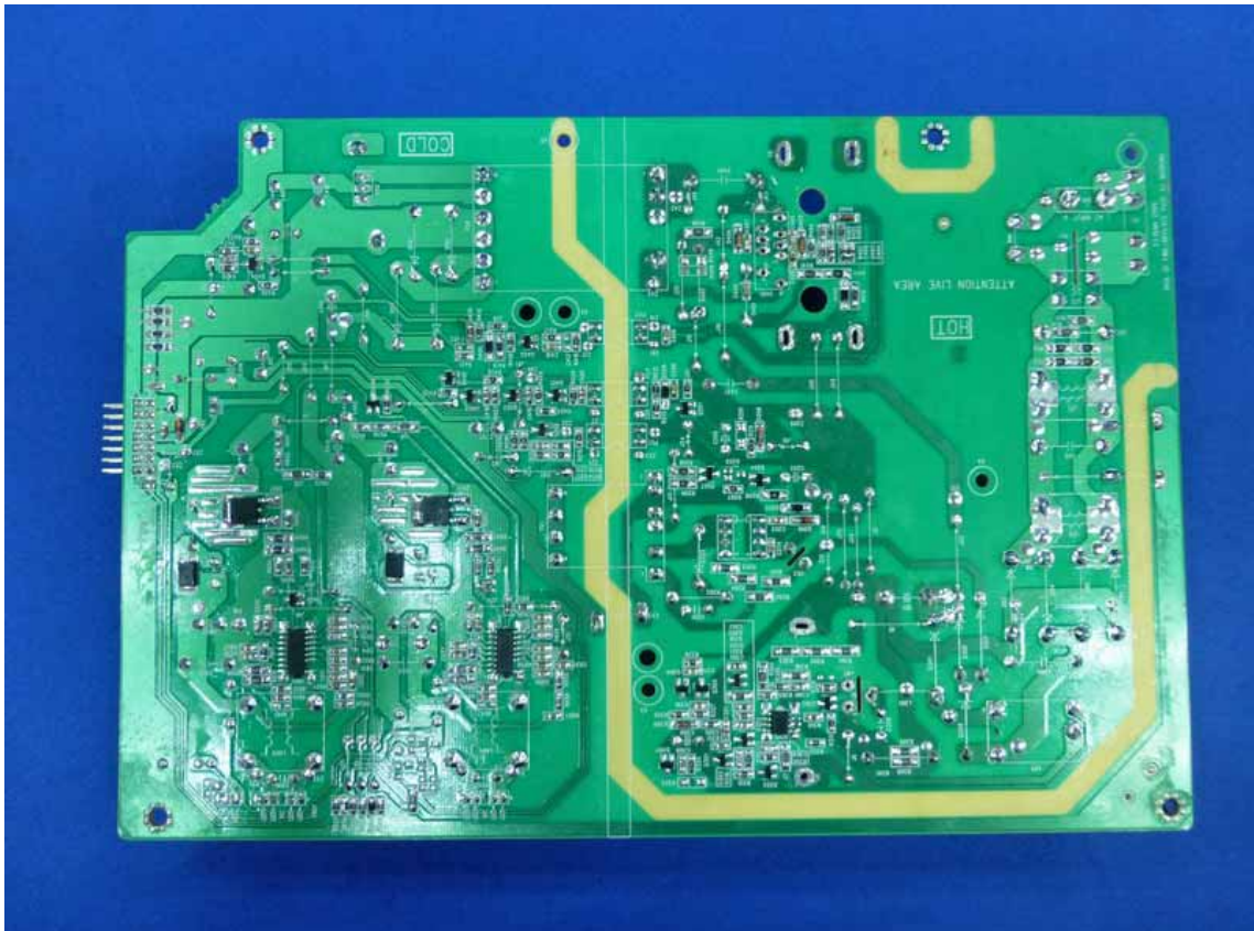
Figure 19 Frontside of the Power Board
